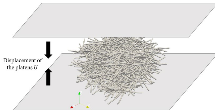
Figure 3.9: Through-thickness compaction of a stack of fiber bundles between two moving platens.
