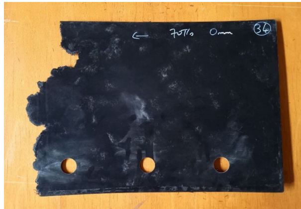
Figure 1.7: Irregular flow front observed by (Oter-Carbonell, 2018).
