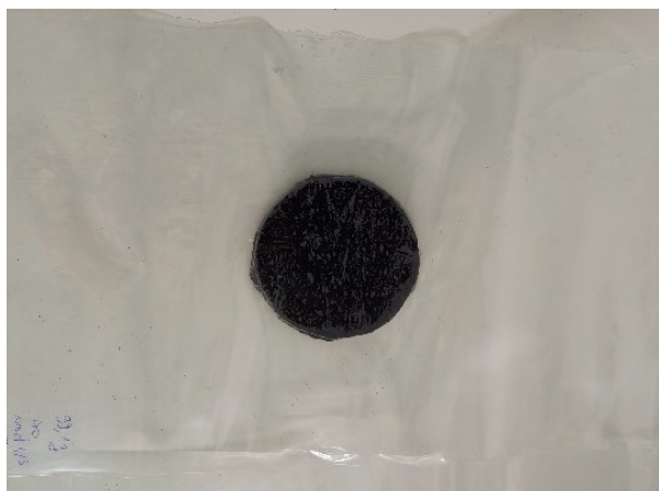
Figure 4.8: SMC circular sample of LF-SMC-30 between polyamide films.
