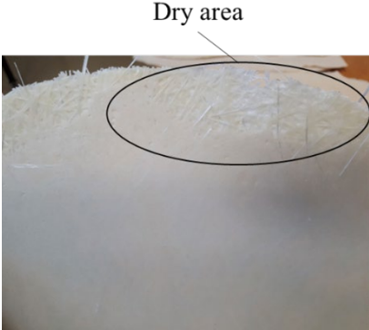
Figure 2.36: Dry area at the flow front.
