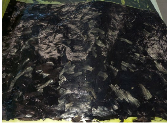
Figure 4.6: Undeformed sheet of CF-SMC-50. The carbon fiber strands are clearly visible from the surface.
