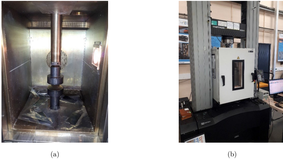
Figure 4.1: Lab-scale experimental compression setup: (a) View of the platens inside the heated room; (b) Outside view with the heated chamber and the Instron testing machine.
