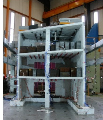
FIGURE 1.11: SMART2013 RC specimen anchored to the AZALEE shaking table.
