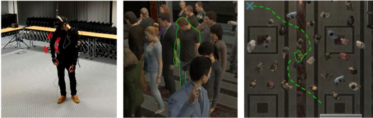
Figure 4.1 – Our objective is to understand whether and to what extent providing haptic rendering of collisions during navigation through a virtual crowd (right) makes users behave more realistically. Whenever a collision occurs (center), armbands worn on the arms locally vibrate to render this contact (left). We carried out an experiment with 23 participants, testing both subjective and objective metrics regarding the users’ path planning, body motion, kinetic energy, presence, and embodiment.
