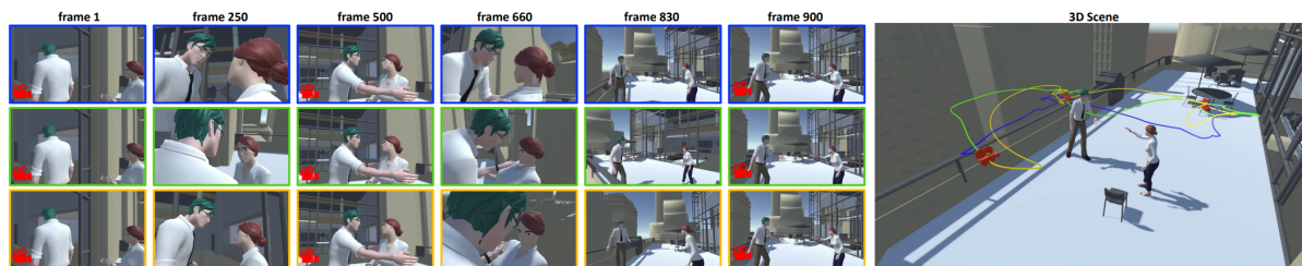
Figure 1.5 – Example of a various sequence of camera motion generated automatically by the technique proposed by Jiang et al. [2021]. Each sequence (blue, green and yellow) is generated with a different behavior while respecting the given constraint, represented by the red camera position and orientation.
