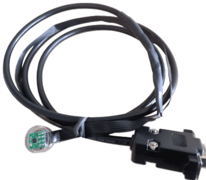
Figure 3.8 – Custom lead for MCG signals acquisition.
