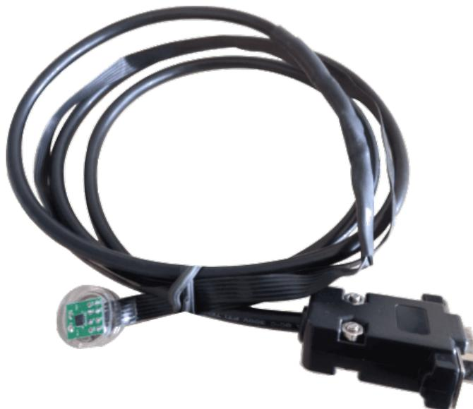
Figure 3.8 – Custom lead for MCG signals acquisition.
