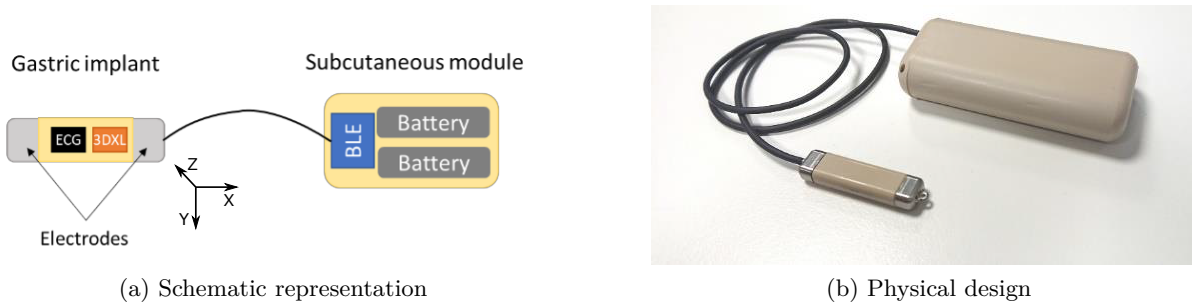
Figure 2.3 – Gastric implant prototype V1.
