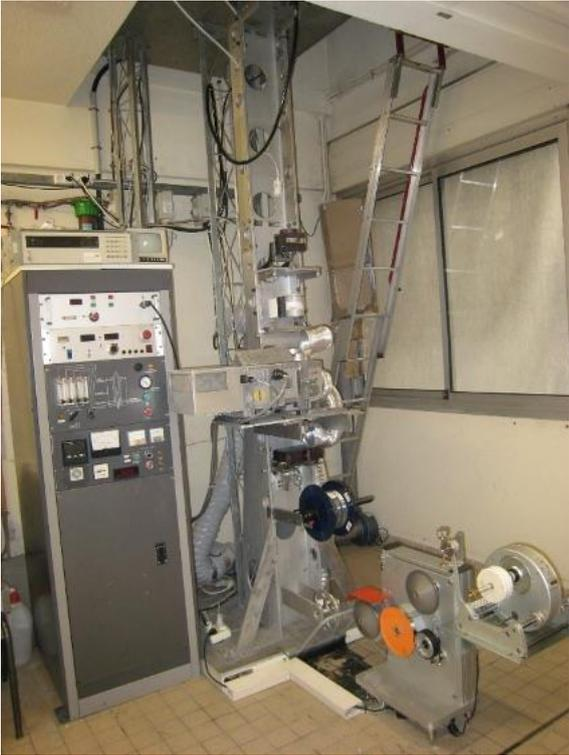
**Figure 1.9** Drawing tower used at the INPHYNI laboratory.
