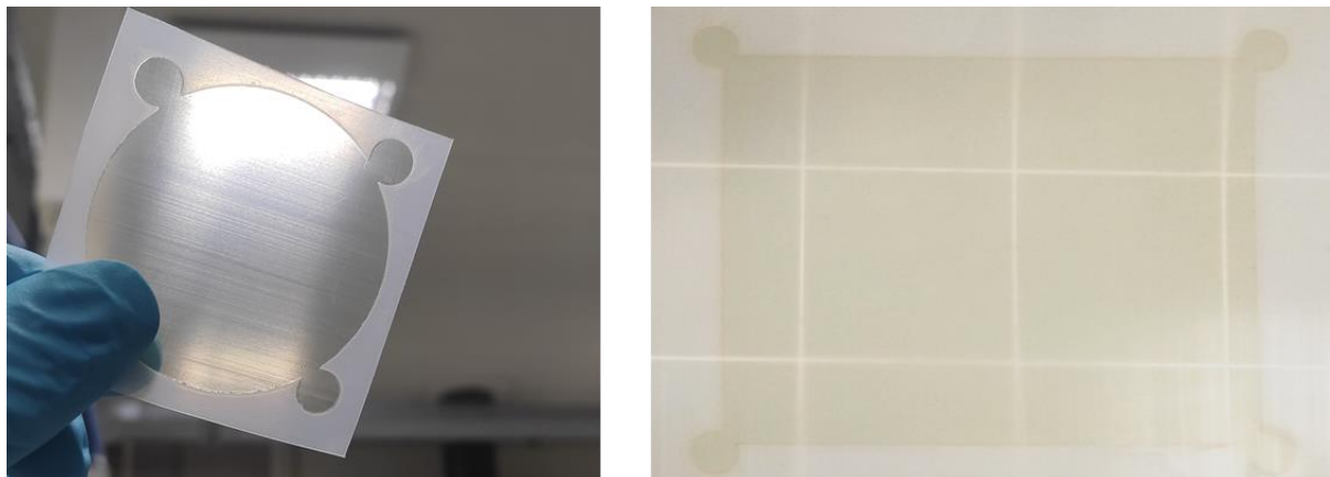
Figure 53 – Two defect-free film samples using two different spacer-mold designs.
