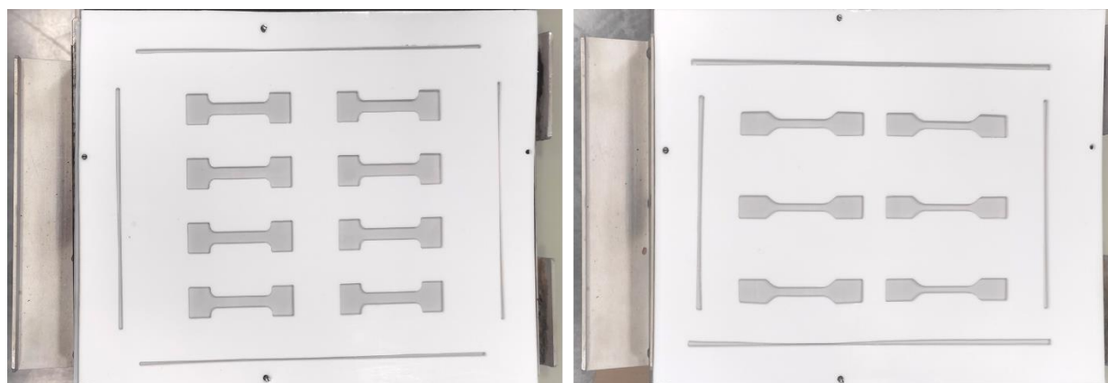
Figure 59 – Left) Thick PTFE mold with 8 dumbbell samples using the simple design. Right) A similar mold using six samples using the standard design. Both designs exhibit protective overflow empty volumes at the edges.
