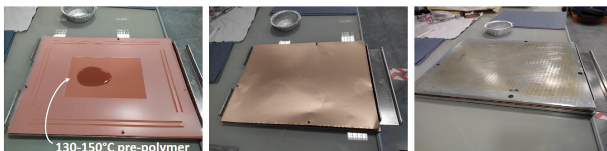
Figure 73 – Layering of the mold system. Left) Press-plates / Copper foil / Mold layer / hot pre-polymer, Middle) Addition of the top copper foil, Right) Entire pressing vessel closed
