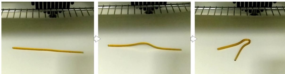
Figure 57 – New permanent shape memory imparted to a previously straight vitrimer piece.
