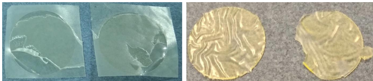
Figure 52 – Left) Adherent samples in the fluorinated unmolding material. Right) Unmolded but deformed samples obtained with 75µm thin PTFE unmolding sheets.
