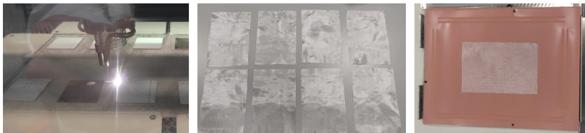
Figure 76 – Left) Cutting process using a CO 2 laser. Middle) Repeatable cut of glass fibers. Right) A fiberglass cloth deposited onto the bottom copper sheet and filling the mold cavity.
