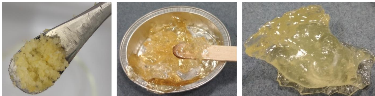
Figure 48 – Left) TBD catalyst as a yellow rubbery solid. Middle) TBD catalysed vitrimer following stirring. Right) Piece of a TBD-catalysed vitrimer including many bubbles trapped during stirring.
