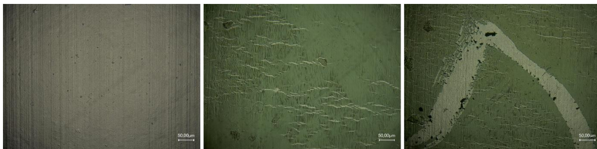
Figure 92 – Left) Surface observation away from the gold electrodes. Middle) Observation in the middle of a gold electrode. Right) Largest gold damage found on a sample
