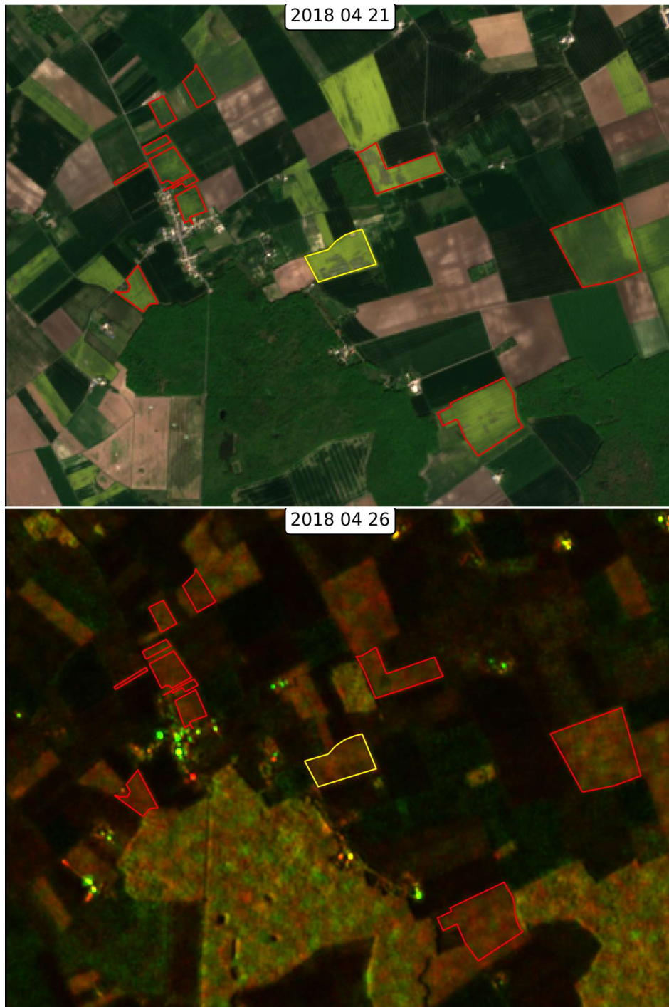
Figure 3.13: Example of a parcel of rapeseed crop (yellow boundaries) where heterogeneity occurs almost during the complete season. Some other parcels show some signs of heterogeneity too. Top: true color S2 image acquired in May, bottom: composite SAR image (green channel is VV polarization and red channel is VH polarization) acquired in May with multi-temporal speckle filtering.
