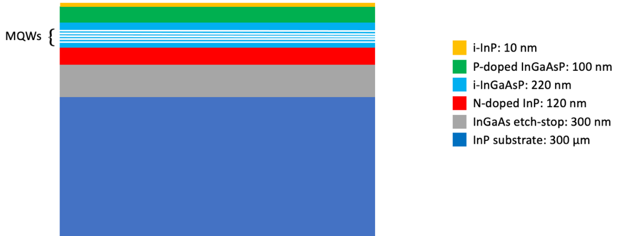
Figure 90: Schematics of the adopted InP-based membrane
