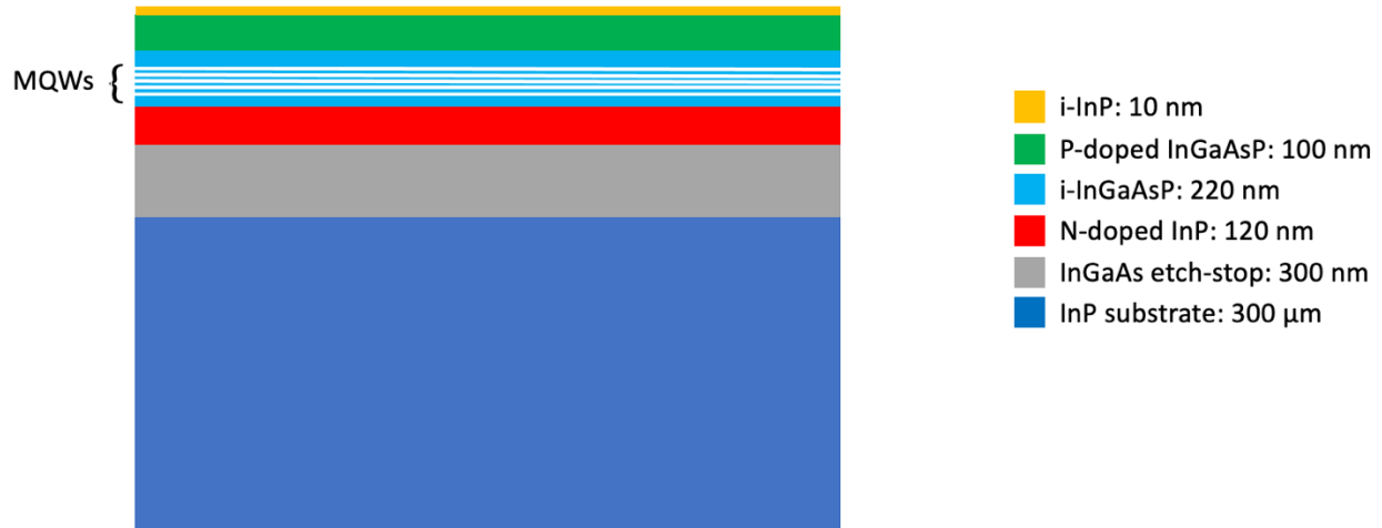
Figure 90: Schematics of the adopted InP-based membrane
