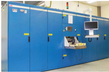
(a) Picture of the test system for IGCTs and diodes at Hitachi ABB Power Grids, Semiconductors
