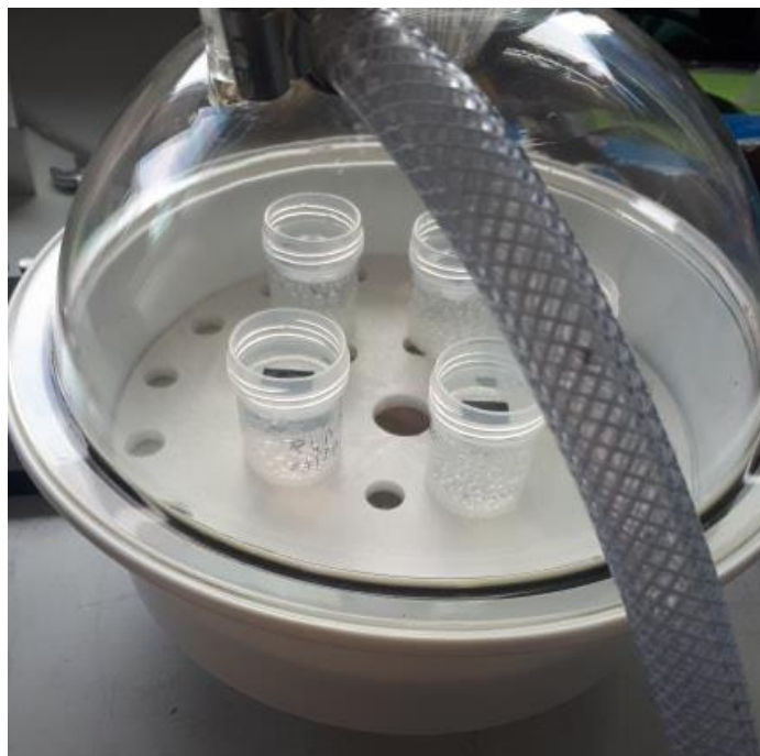
Fig 3. 30: GDLs inside a chamber connected with a vacuum pump.
