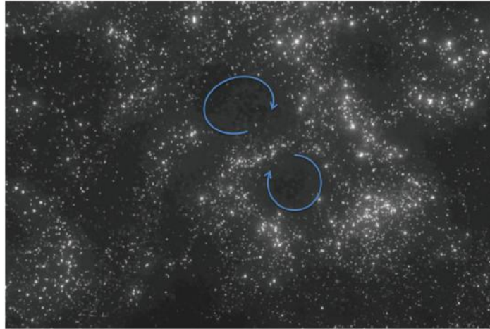
Figure 6.2: Laser-sheet image of particles in homogenous turbulence illustrating inertial clustering. From [316].
