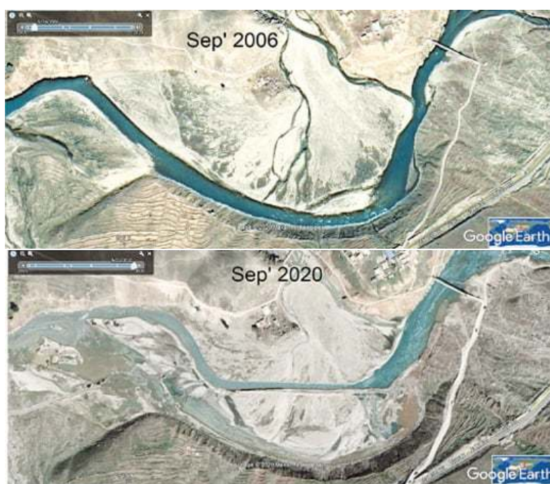
Figure 2.36: Kunhar River diverted at Sohach for gravel and sand mining (above: Sept 2006; below: Sept 2020) | Dawn GIS.
