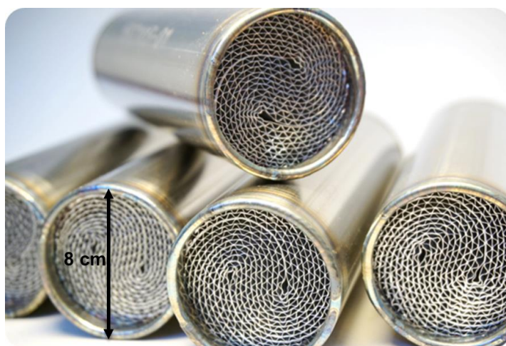
Figure 1-14: Honeycomb cylinders used in the catalytic methanation reactor of the Falkenhagen plant, adapted from [183]
