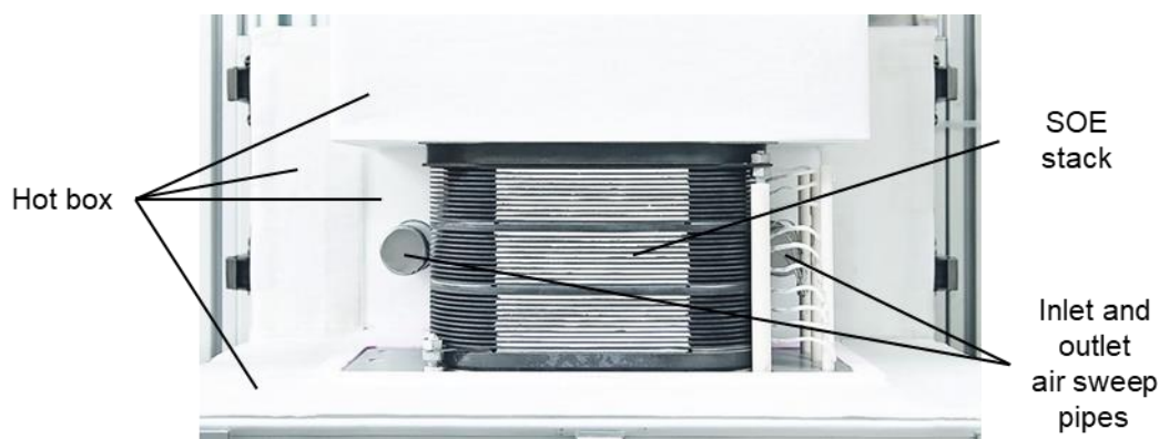
Figure 1-11: Hot box configuration of the company Sunfire, adapted from [90]
