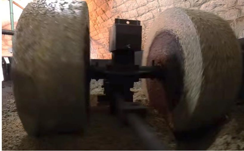
Photo 9: A traditional olive oil stone mill in the town of Btaaboura in Al Koura North Lebanon being used to grind olives into a paste prior to pressing. Photo credit: Anthony Rahayel YouTube channel 11
