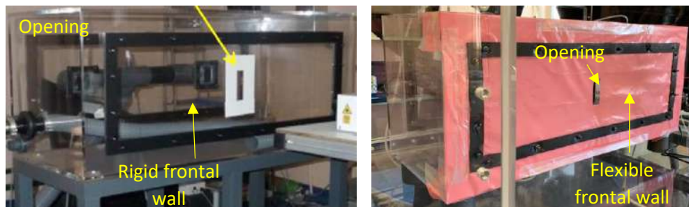
Figure 3-6 The enclosure with rigid frontal wall (left) and flexible frontal wall (right)
