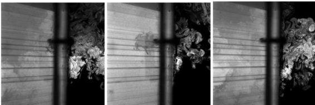
Figure 0-4 Visualizations fields in the median vertical plane in the opening of the enclosure with its rigid frontal wall and with a counter-current internal disturbing jet
