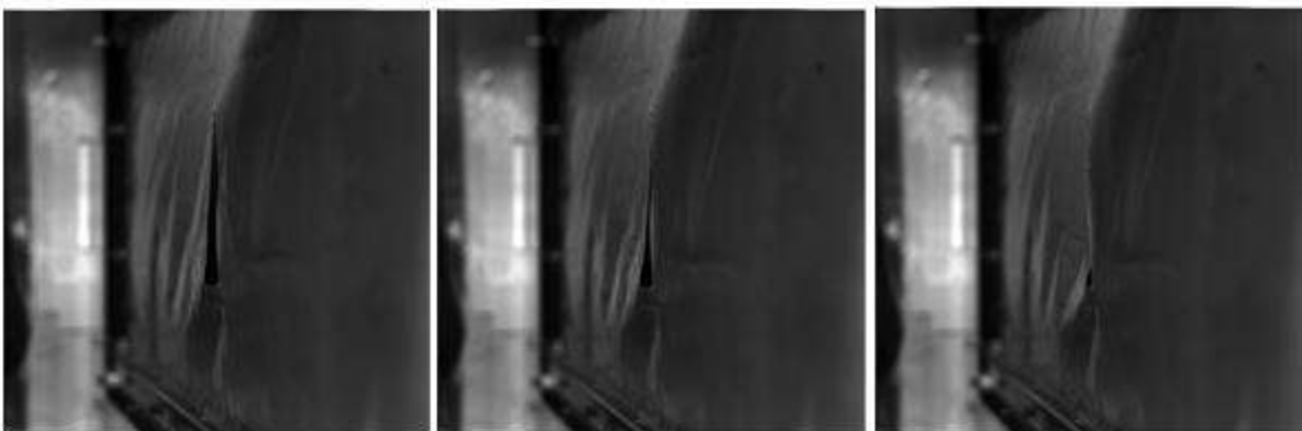
Figure 0-6 Visualizations fields in the median horizontal plane in the opening of the enclosure with its flexible frontal wall and with a counter-current internal disturbing jet, inside the enclosure
