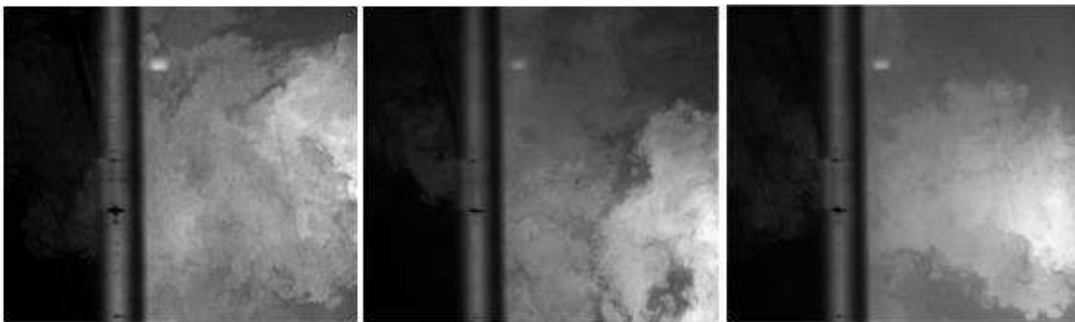
Figure 0-3 Visualizations fields in the median horizontal plane of the opening of the enclosure with its rigid frontal wall and with a counter-current internal disturbing jet
