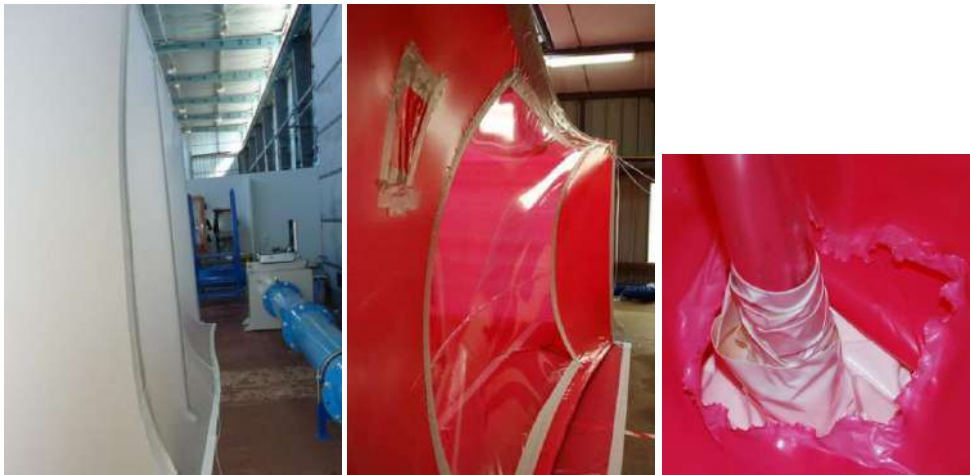
Figure 1-4 Mechanical strength tests on flexible airlock with negative pressure (from left to right): -10 Pa, -40 Pa, -100 Pa (Ducos, 2016)
