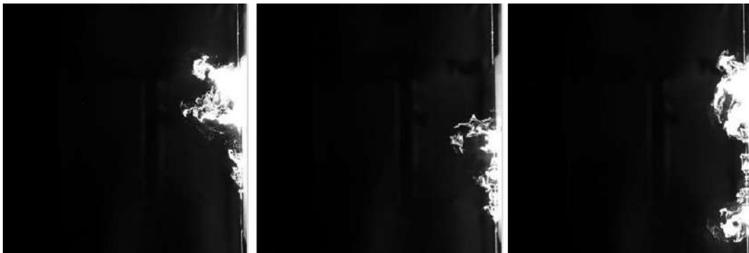
Figure 1-16 Laser visualizations of the vertical plane outside the enclosure under the influence of an external parietal disturbance, showing the tracer backflow near the opening (Kaissoun, 2018)
