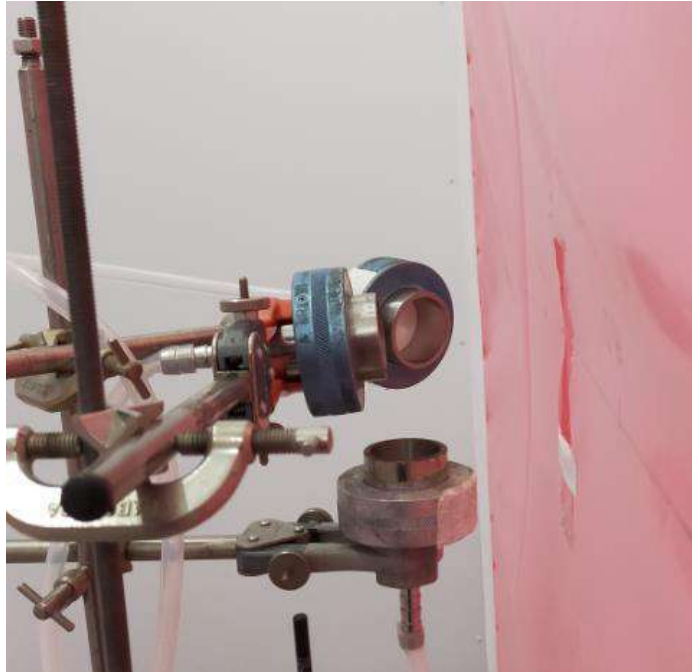
Figure 5-5 Three samplers added near the opening of the airlock
