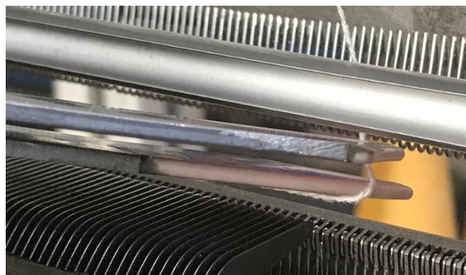
Figure 5.21: Wrap angle of the thread on the edge of the blade from the rotor
