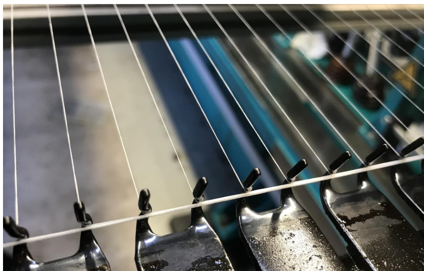
Figure 4.3: Inlay-yarns placed inside the hooks from the transportation chain
