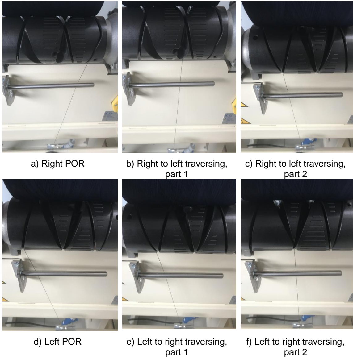
Figure 3.5: Yarn traversing in the grooved roller of a winding machine: a) to c) from the right point of return (POR) to the left side and d) to f) from the left point of return (POR) to the right side of the machine.
