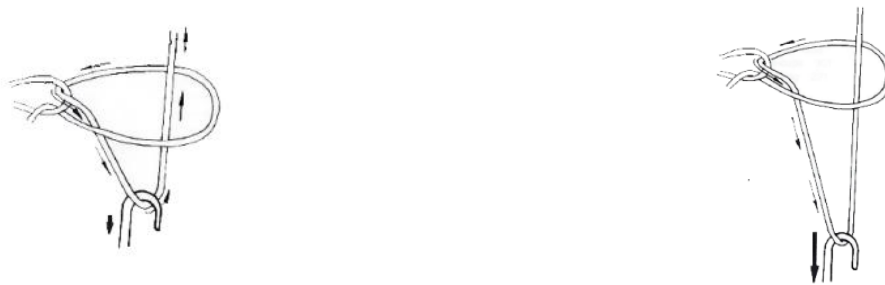
Figure 4.1: Loop formation showing the 'robbing-back' and yarn tensile forces on the needles for the warp knitting process from left to right 15
