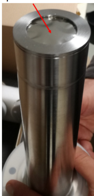
25 \mu\text{m} stainless steel Window
