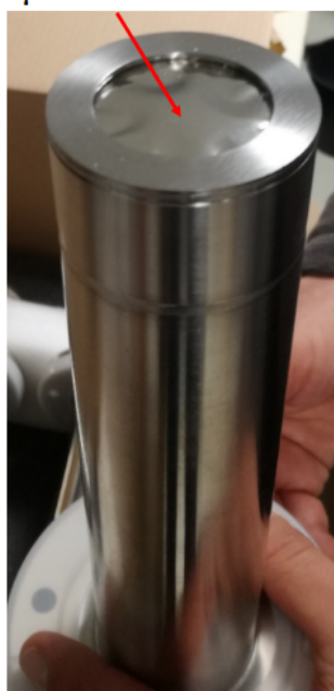
25 \mu\text{m} stainless steel Window
