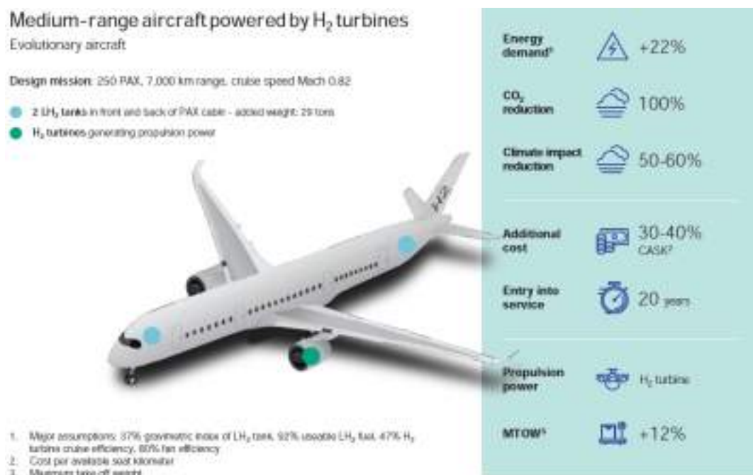
Figure 1.8: Projected feasibility and cost of a medium-range aircraft powered by H 2 turbines by McKinsey & Company in 2020 [6].
