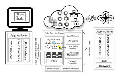
Figure 4.9: Service Oriented System Architecture of UAV [160]
