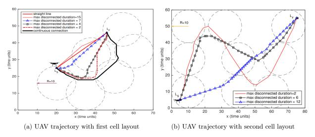
Figure 4.4: UAV trajectory for two different layouts with varying discontinuity threshold [147]
