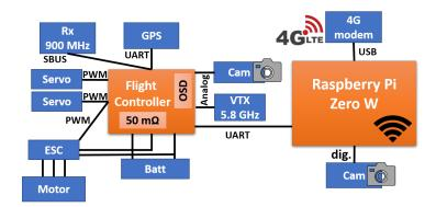
Figure 4.12: Schematic of the avionics components in [172]
