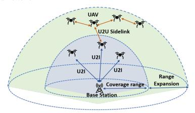
Figure 3: UAV-to-UAV links using Sidelink
