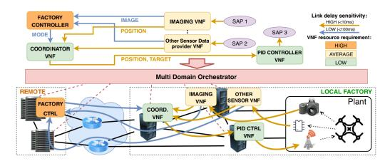
Figure 4.7: Deployment on multi-domain UAV services [153]
