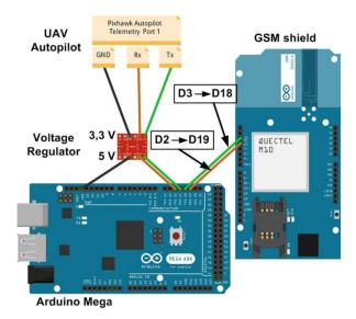
Figure 4.13: High level shematics of the prototype setup in [174]
