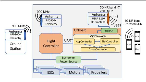
Figure 2.4: Design and Schematics of UAV-BS prototype
