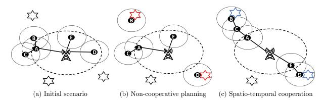
Figure 5.6: Dynamic aerial network formation and coverage constraints
