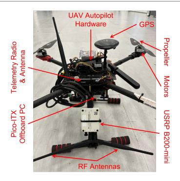
Figure 2.3: UAV-BS Prototype Platform
