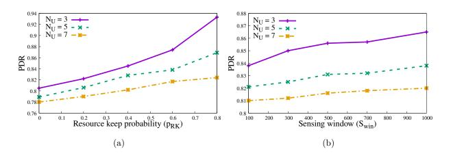
Figure 5.16: Chain Scenario - PDR index (a) by varying  $p_{RK}$ , (b) by varying  $S_{win}$ .
