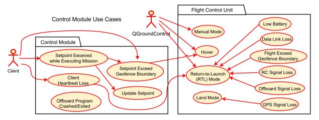
Figure 2.5: DroneController flight-safe implementation
