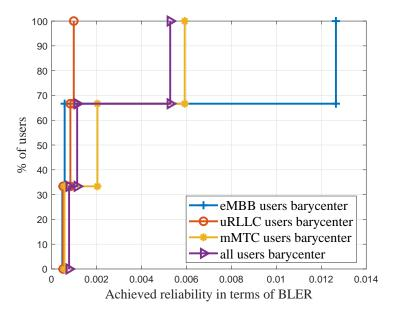
Figure 3.9: Improved reliability performance resulted from placing UAV-BS at uRLLC barycenter vs. other barycenters
