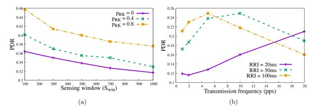
Figure 5.18: The evaluation of the UAV swarm scenario varying both  $p_{RK}$  and  $S_{\text{win}}$  is depicted in Figure 5.18a. The impact of the RRI parameter on the performance is shown in Figure 5.18b.
