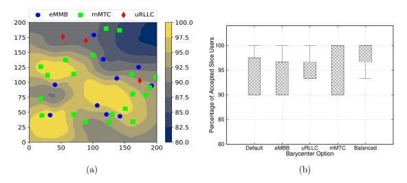
Figure 3.8: (a) Heatmap denoting the percentage of accepted slice users according to positioning of UAV-BS in 200  $m \times 200$  m. (b) Box-and-whisker plot showing percentage of accepted users for different barycenter choices of positioning UAV-BS.
