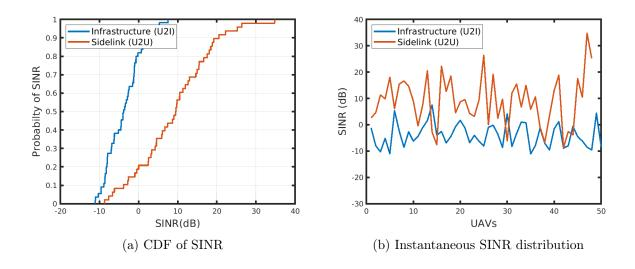
Figure 5.4: Coverage comparison of sidelink (U2U) with infrastructure (U2I) links
