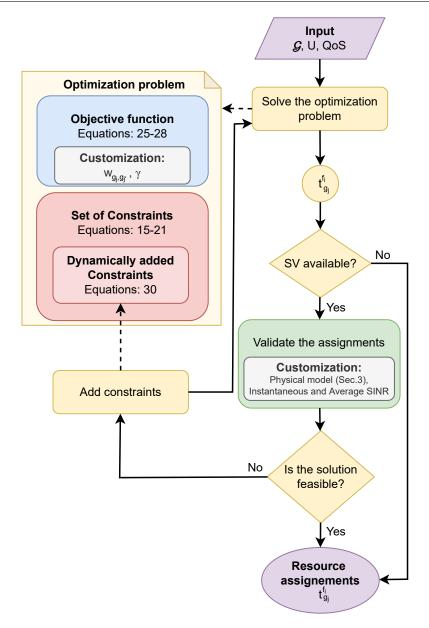
Figure 3.4: EASIER: the execution flow
