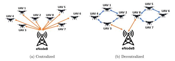
Figure 5.1: Cellular-connected UAV swarm architecture
