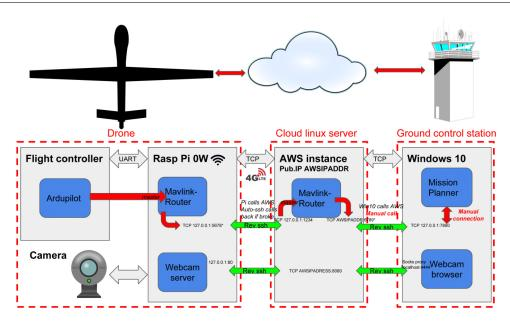
Figure 4.11: Prototype design and configurations in [172]
