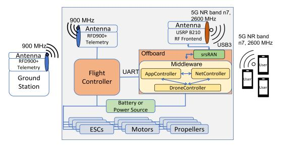
Figure 2: Design and Schematics of UAV-BS prototype
