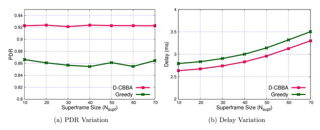
Figure 5.11: PDR and Delay varying with superframe size  $(N_{\text{supf}})$ .
