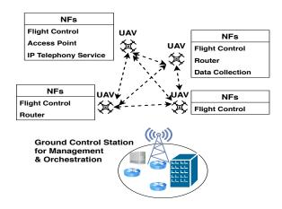
Figure 4.6: UAVs with diverse network functions
