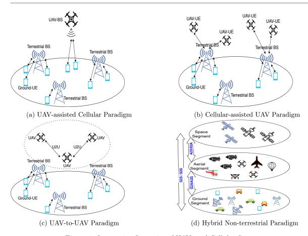
Figure 1: Integration Synergies of UAVs and Cellular System
