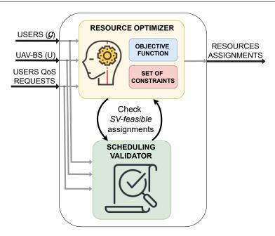
Figure 3.3: EASIER: modular components and architecture
