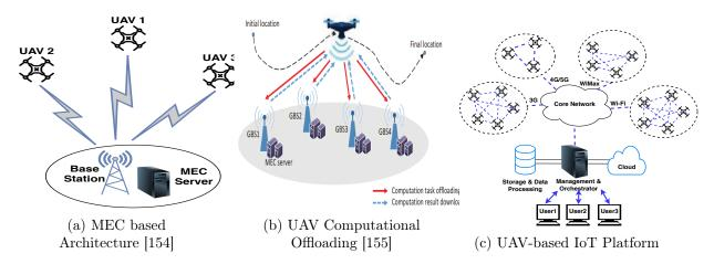
Figure 4.8: Network Architectures of Cellular-connected UAV
