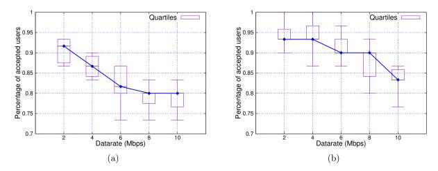
Figure 3.6: Percentage of accepted eMBB users w.r.t. varying data rate for (a) SV-AVG and (b) SV-INST
