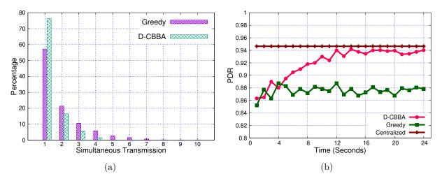
Figure 5.10: (a) Percentage of simultaneous transmissions for Greedy and D-CBBA, (b) Comparison of the algorithm convergence time.
