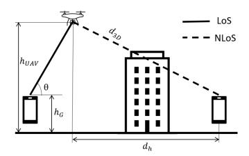
Figure 2.1: Geometry of Air-to-Ground propagation
