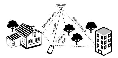
Figure 2.2: Air-to-ground propagation phenomena
