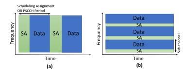
Figure 5.2: Resource Pool Structure: Mode (a) 1,2 (b) 3,4
