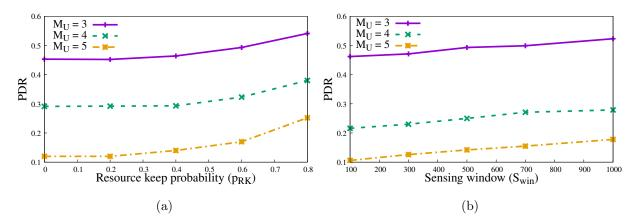
Figure 5.17: Grid Scenario - PDR index (a) by varying  $p_{RK}$ , (b) by varying  $S_{win}$ .
