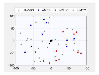
Figure 3.5: An example deployment with one UAV-BS positioned at origin (0,0) flying at 50 meters altitude in  $200 \ m \times 200 \ m$ . Ground UEs of three slice service types (10 eMBB, 10 uRLLC and 30 mMTC) are deployed randomly within the area.
