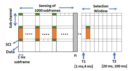
Figure 5.13: Mode-4 Sensing-based Semi Persistent Scheduling
