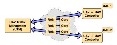
Figure 6.3: High level architecture of 3GPP Release 16 work on remote identification of UAS
