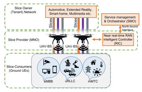
Figure 3.1: RAN Slicing of UAV-assisted 5G network.
