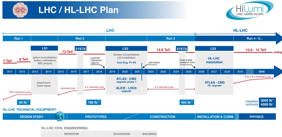
Figure 1.1: Timeline of the LHC upgrade to high-luminosity (January 2022).
