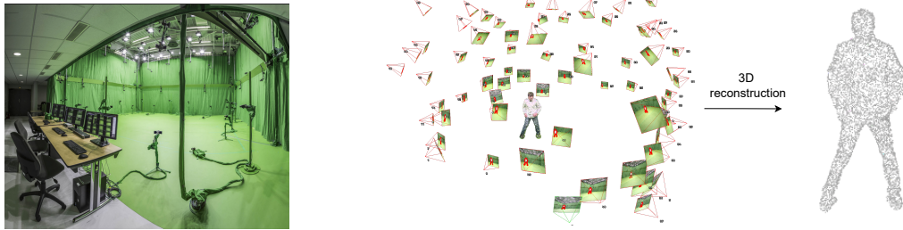
Figure 1.1: Left : picture of the Kinovis multi-view platform. Right : Acquisition pipeline, an actor is filmed under multiple angles by 68 RGB cameras. A 3D point cloud is then computed from the images using the 3D reconstruction algorithm proposed in [1].
