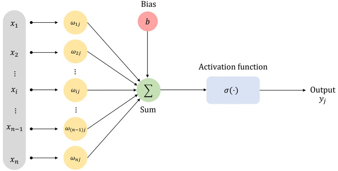
Figure B.1: Illustration of an artificial neural network
