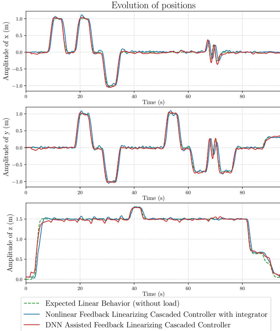
Figure V.6: The spatial position of the quadrotor with the unknown suspended payload over the experimental test scenario.
