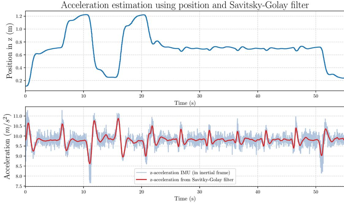
Figure II.13: Example of Savitsky-Golay filtering for getting second order derivative. The first subplot is the  $z$  position of the quadrotor obtained from the VICON. It is used to obtain the red curve in the second subplot.
