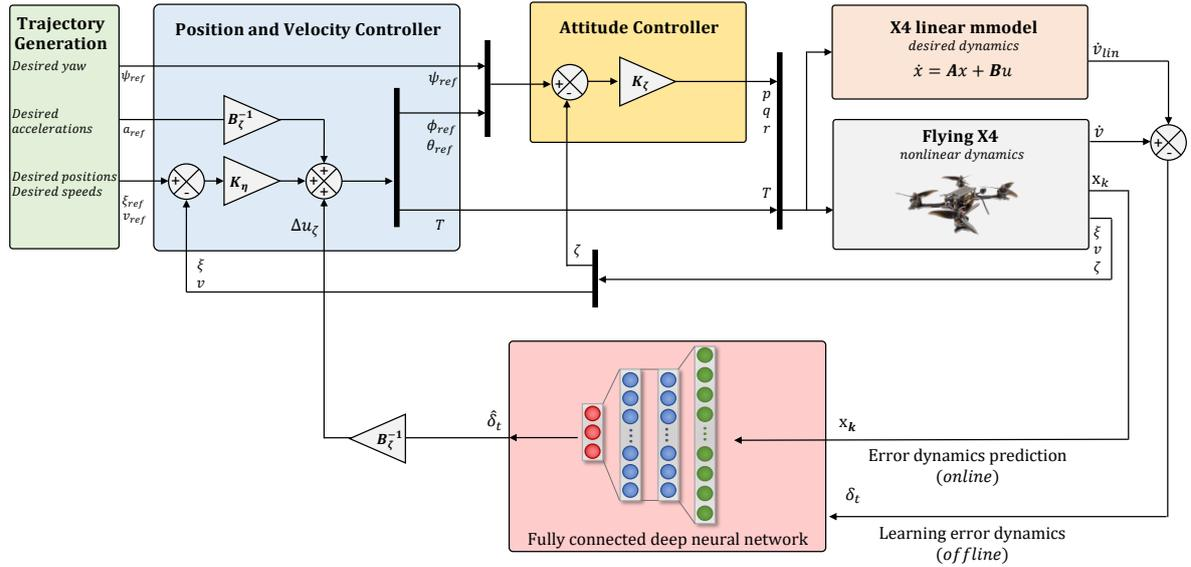
Figure III.5: DNN-enhanced linear controller architecture
