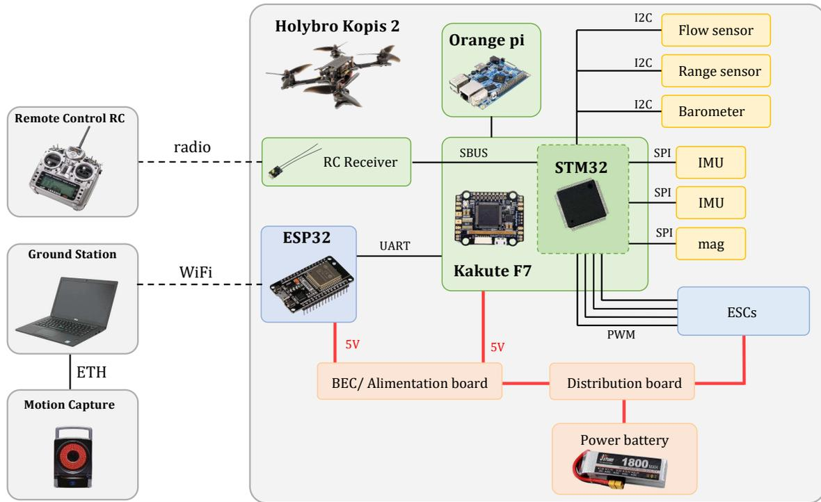
Figure II.2: The Holybro Kopter 2 hardware configuration.
