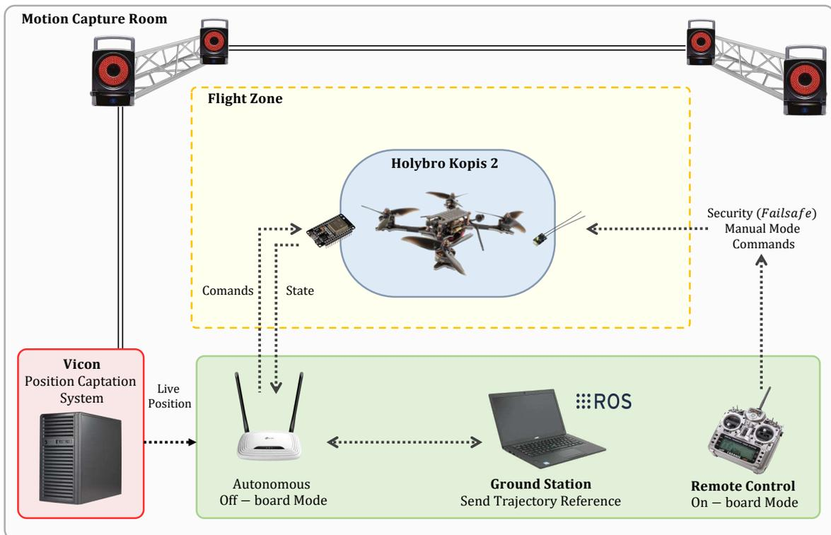
Figure II.3: Schematic representation of the motion capture room.
