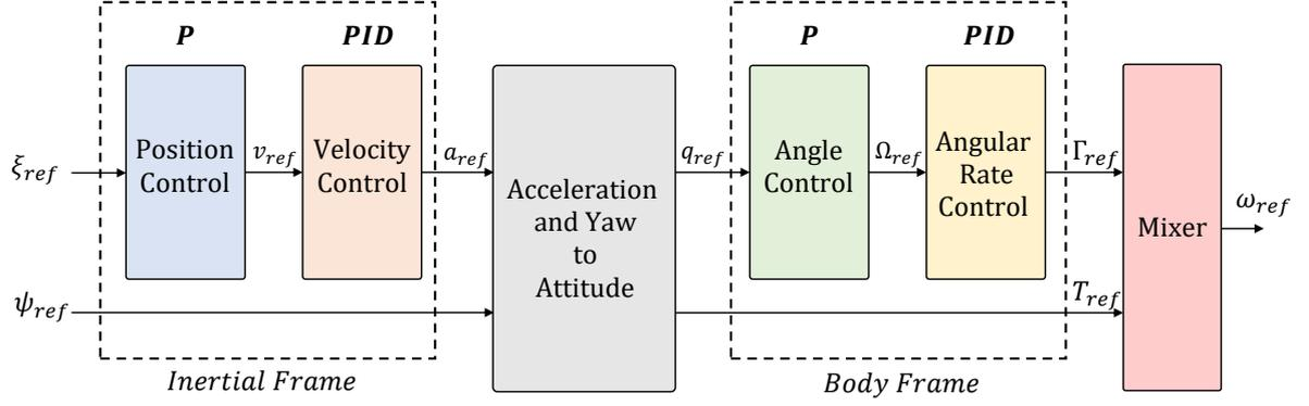
Figure II.7: Common cascaded control architecture for quadrotor.
