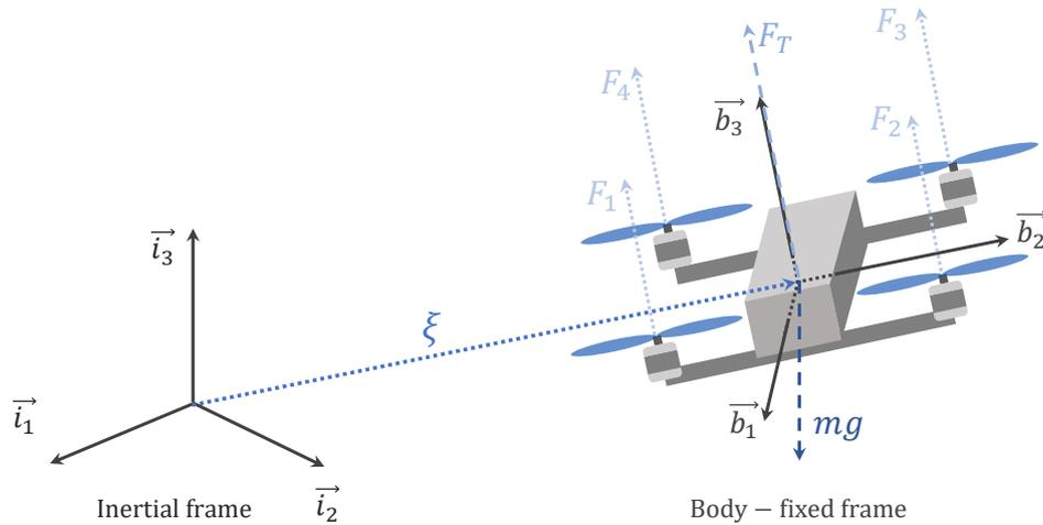
Figure I.8: Quadrotor mains forces after making assumptions.
