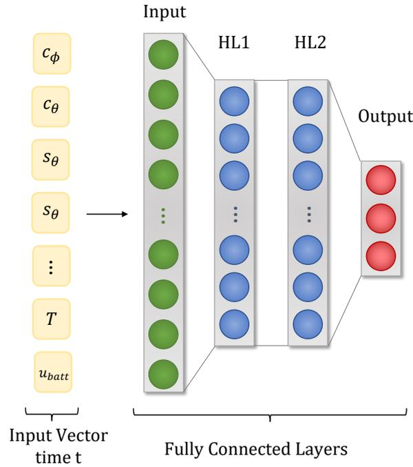
Figure III.4: The deep neural network structure: a feed-forward DNN, composed of  $N_l$  hidden layers of  $N_u$  units, using ReLU as activation functions.
