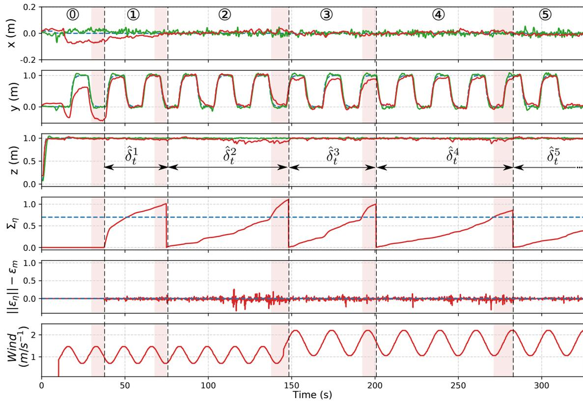
Figure IV.6: The event-based neural learning strategy experimental test: back and forth motions in front of a sinusoidal varying wind. Red areas represent learning and re-learning process. For  $x$ ,  $y$  and  $z$ , the red curve is the result with the event-based neural learning strategy. The green curve is the obtained result with the PID along with disturbance observer. The blue one is the expected linear behavior with the linear PD controller only.
