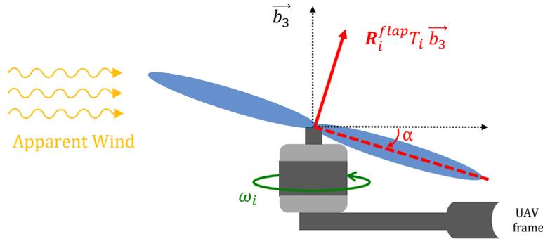
Figure I.7: Illustration of the blade flapping effect.
