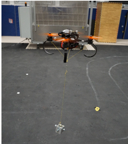
Figure V.1: An example of a suspended payload transportation using a quadrotor.
