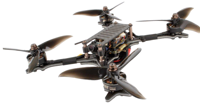
Figure II.1: The Holybro Kopis 2 quadrotor.
