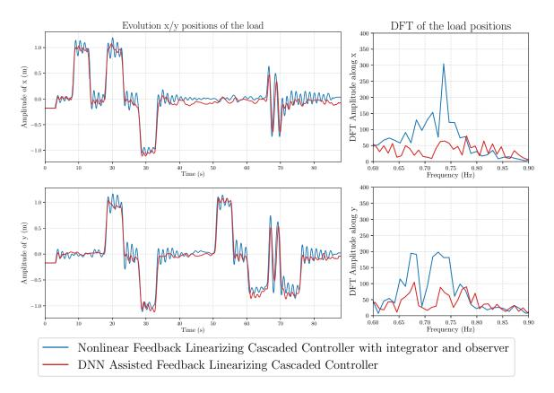
Figure V.9: Experimental payload positions during transportation test flight and DFT (modulus) of the signals around load oscillations.
