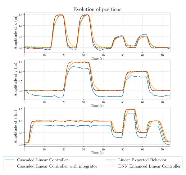
Figure III.8: Evolution of the quadrotor positions for each controller, in real flight test using our motion capture room.
