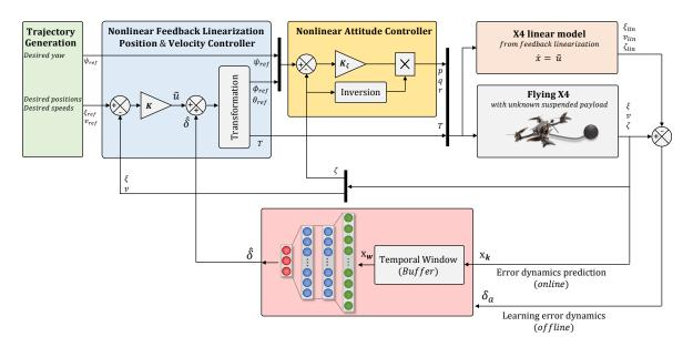
Figure V.3: The DNN-assisted nonlinear cascaded control to perform trajectory tracking with an unknown suspended payload.
