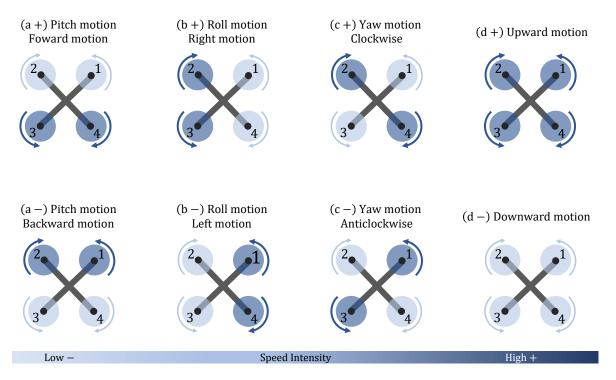
Figure I.2: X4 - Quadrotor motion description.
