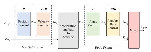
Figure II.7: Common cascaded control architecture for quadrotor.
