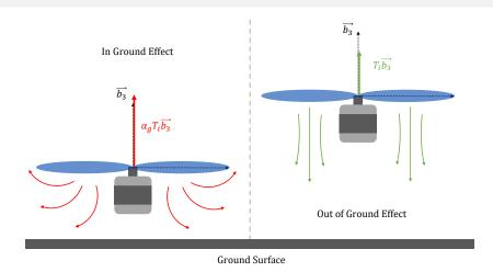
Figure I.6: Illustration of the ground effect.
