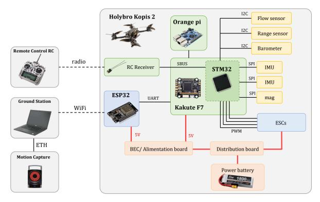
Figure II.2: The Holybro Kopis 2 hardware configuration.
