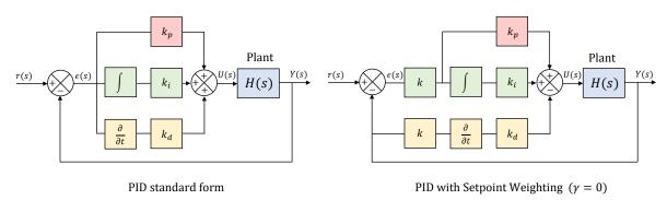
Figure II.9: Different PID architectures. (Left) Standard PID form. (Right) PID with weighting setpoint, the weighting is set to  $\gamma = 0$ , meaning the derivative operate only on the feedback.
