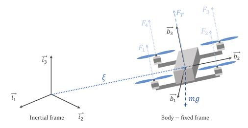
Figure I.8: Quadrotor mains forces after making assumptions.
