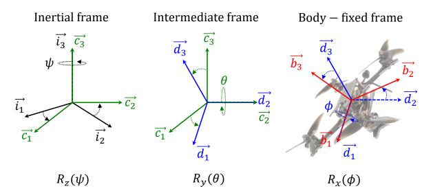
Figure I.3: Illustration of the frames representation using Tait-Bryan angles. The inertial frame on the left, intermediate frames in the middle and the body fixed frame, on the right.
