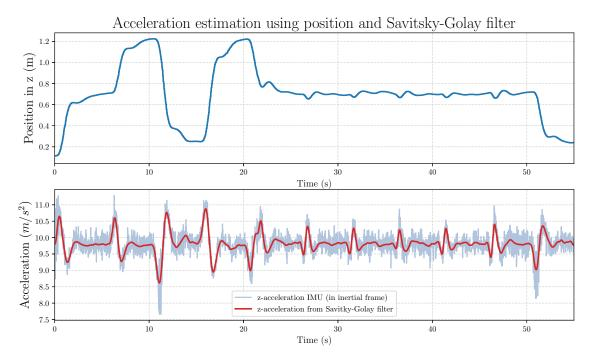
Figure II.13: Example of Savitsky-Golay filtering for getting second order derivative. The first subplot is the z position of the quadrotor obtained from the VICON. It is used to obtained the red curve in the second subplot.
