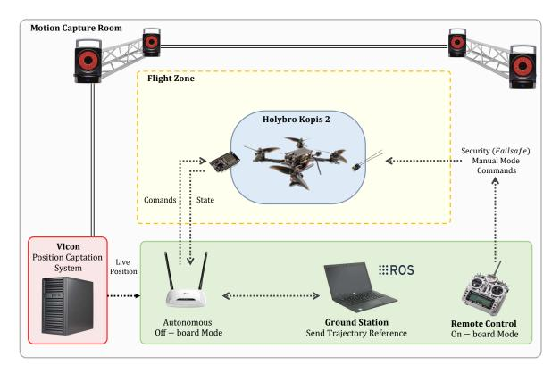
Figure II.3: Schematic representation of the motion capture room.
