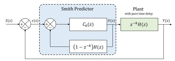
Figure II.10: Smith predictor block diagram.
