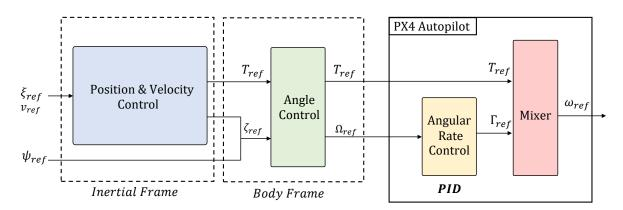
Figure II.8: Proposed general control architecture.
