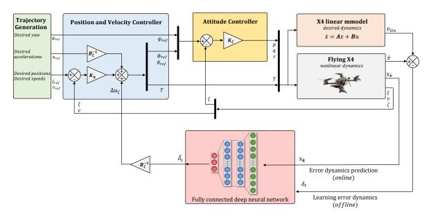
Figure III.5: DNN-enhanced linear controller architecture
