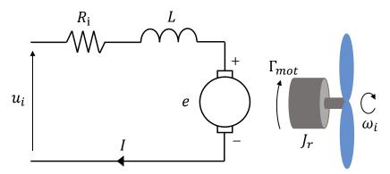
Figure I.4: Brushless motor equivalent mono-phase circuit.
