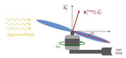
Figure I.7: Illustration of the blade flapping effect.
