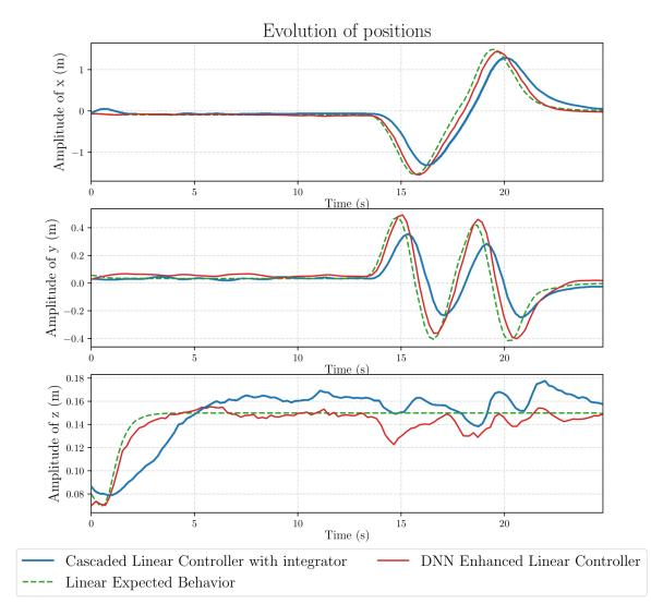
Figure III.9: Evolution of quadrotor positions for the linear cascaded controller versus the DNN-enhanced linear controller in a near -ground scenario.
