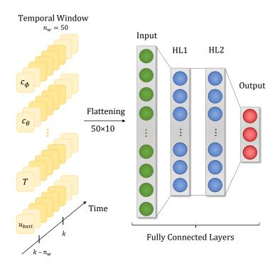
Figure V.4: The windowed deep neural network architecture.
