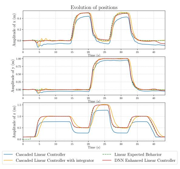
Figure III.7: Evolution of the quadrotor spatial positions for the three controllers in ROS/Gazebo simulation environment, for the test case scenario.
