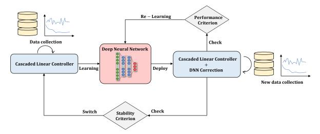
Figure IV.1: The proposed event-based neural learning strategy. At starting, an initial cascaded linear controller is used. It is enhanced with DNN learning after data collection. Two criteria are used to ensure both stability and flight tracking performance. If the stability is faulty, the control is switched to the initial controller.
