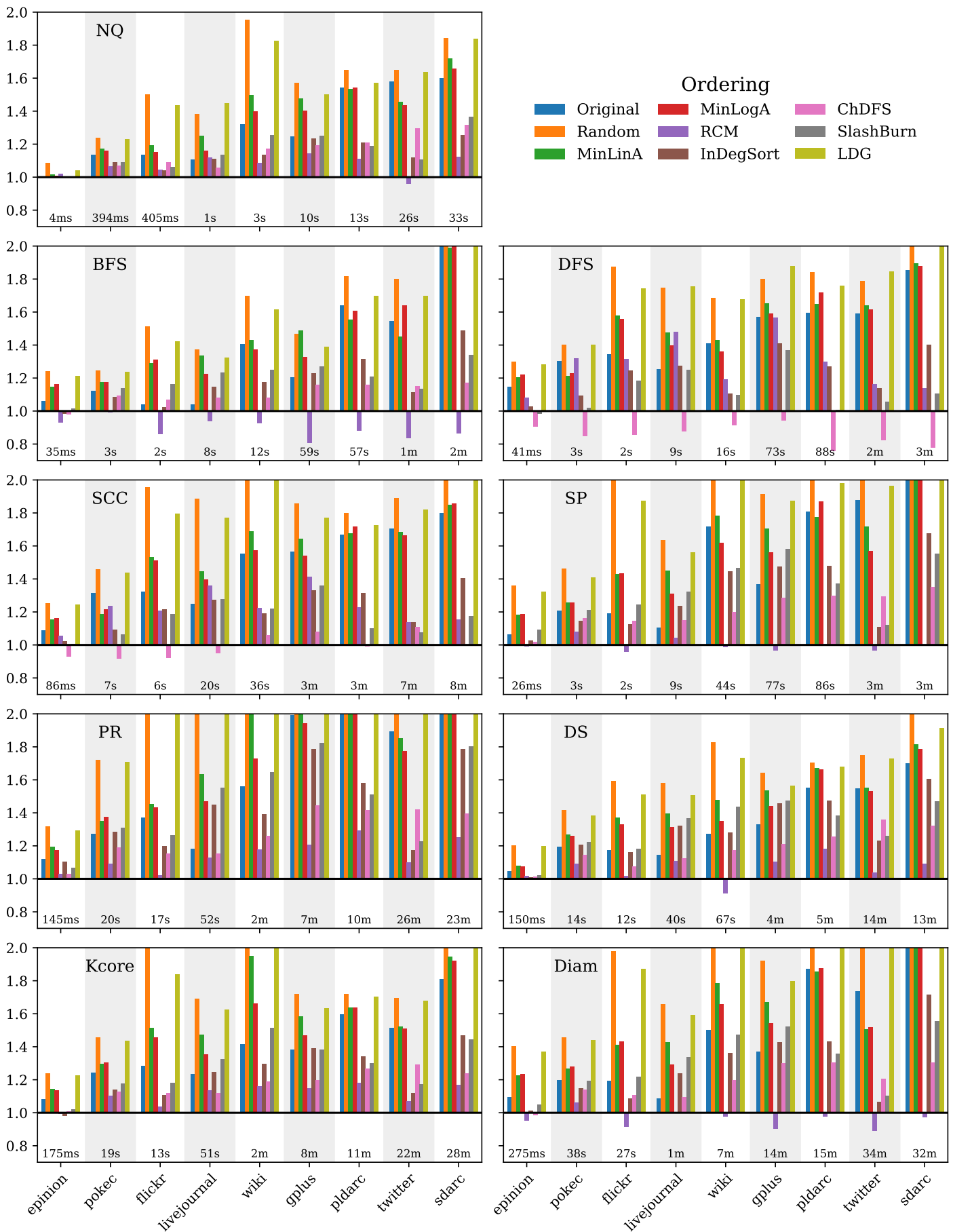
Figure 4.5: Speedup of Gorder. For each algorithm and each dataset, we display the absolute runtime for Gorder. Bars represent the relative time of all other orderings compared to this reference. For readability, the y-axis is cut above factor 2, but values go as high as 3.7. This figure can be compared to Figure 9 in Wei et al. [2016]. Another visualisation is show in supplementary figure 4.6.
