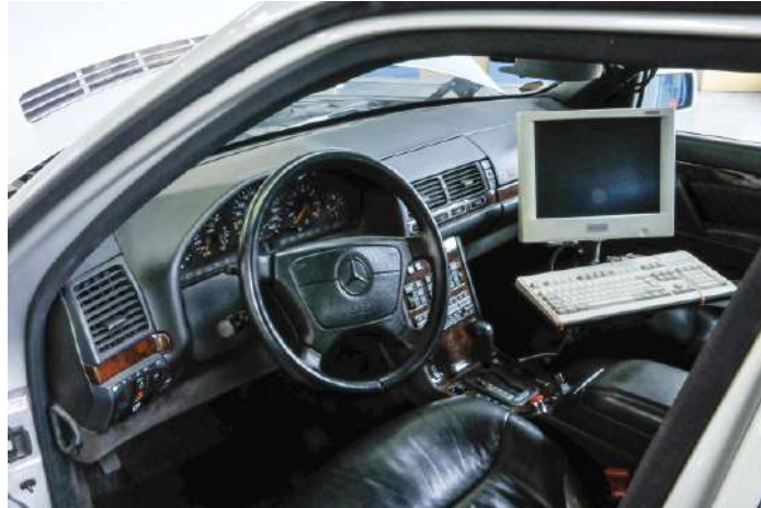
FIGURE 1.1: Interior of the VaMP driverless car [Mercedes-Benz, 2016], one of the first actual autonomous car that completing in 1995 a 1,758 kilometres (1,092 miles) trip in (almost) complete autonomy
