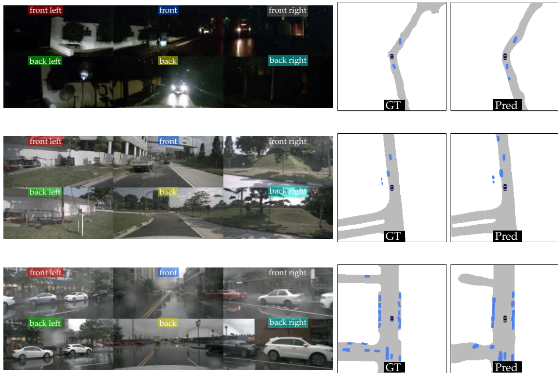
FIGURE 4.2: Qualitative results on complex scenes. We show the six camera views surrounding the vehicle along with segmentation ground truth for reference. Vehicles are shown in blue and driveable area in gray. Vehicles and driveable area predictions are from two different models trained independently for their respective ground-truth, the predictions are then merged for visualization purpose. The ego vehicle is located in the center and facing upwards. Predictions of both driveable area and vehicle segmentation are thresholded at 0.5 for visualization purpose.
