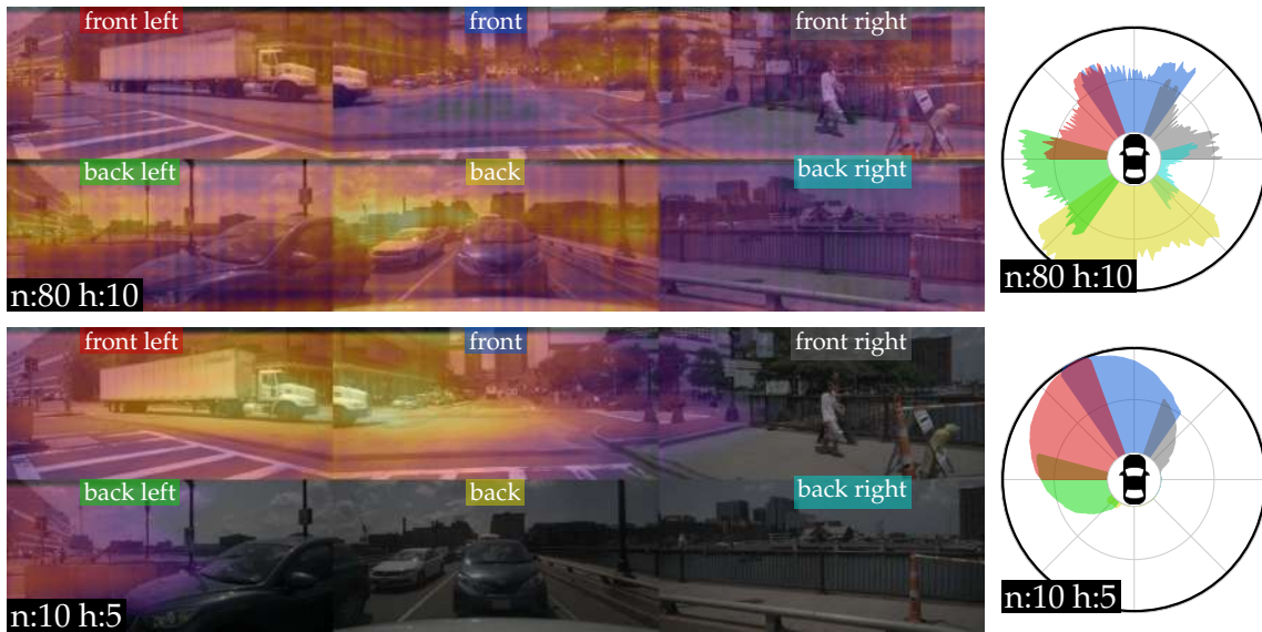
FIGURE 4.5: Input-to-latent attention study — influence of the input embedding. Analysis of attention maps for two networks trained with different input embeddings. Top row is with ‘Fourier + Cam. idx’ and bottom row is with our proposed ‘Cam. rays’ embedding. The attention for one attention head and one latent is shown on the left superimposed with RGB images. The polar plots represent the directional attention intensity for one attention head with one latent vector. The radial distance is proportional to the attention level and shows the directions the network attends to the most.
