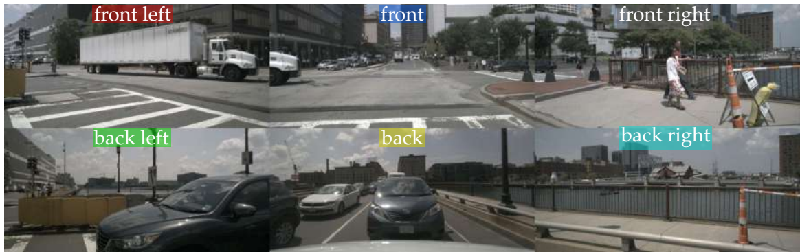
FIGURE B.1: Six input camera images coming from the 360-degree camera rig of nuScenes. Note the small overlaps between views, e.g., the front of the white truck is both seen in the front-left and front cams.
