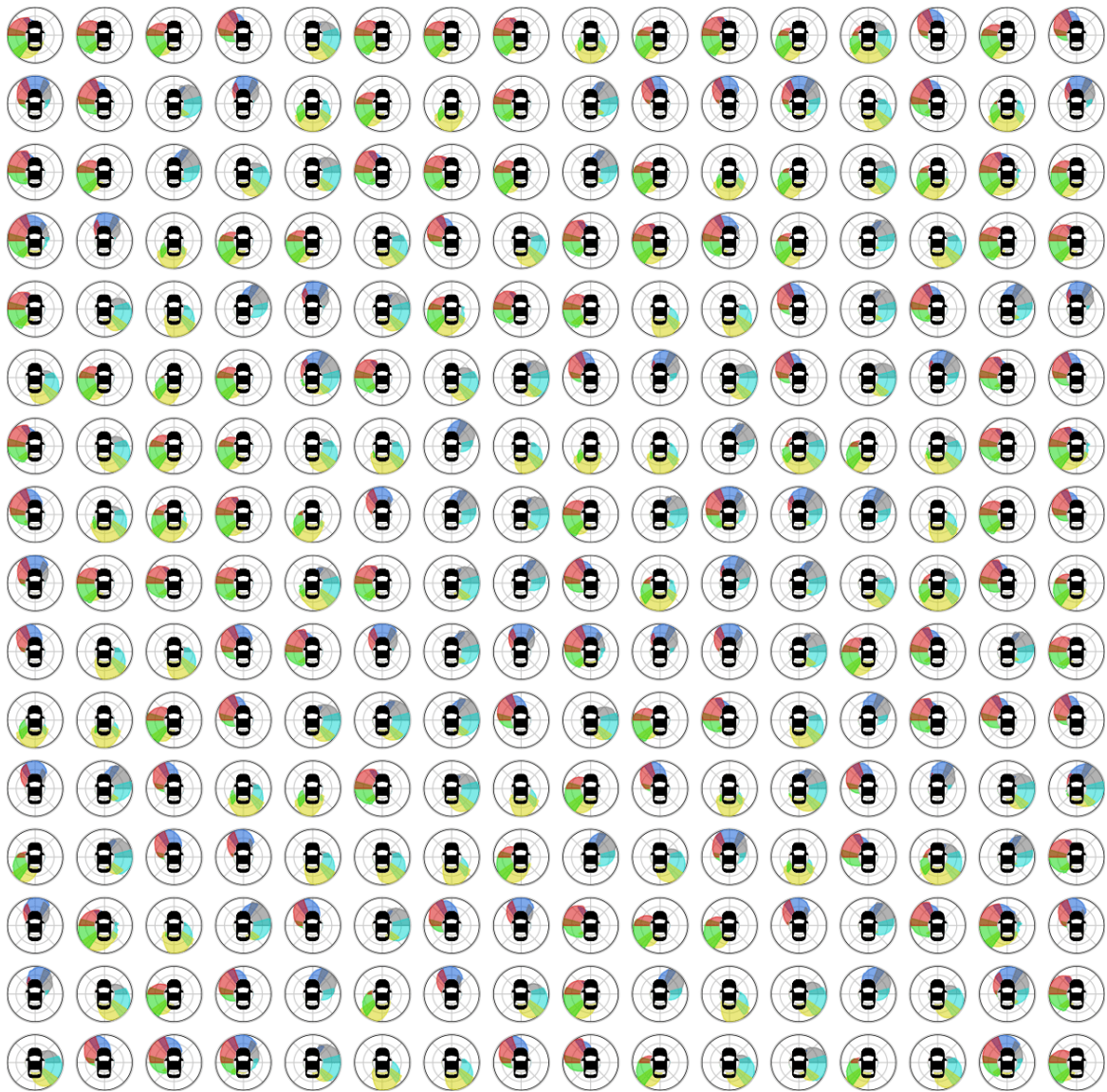
FIGURE B.5: Input-to-latent attention study — all the latent vectors for an attention head. These polar plots represent the directional attention intensity of the 256 latent vectors for a randomly chosen attention head (head #4). As shown in fig. B.2 , one attention head generally covers the full scene over the latent vectors.
