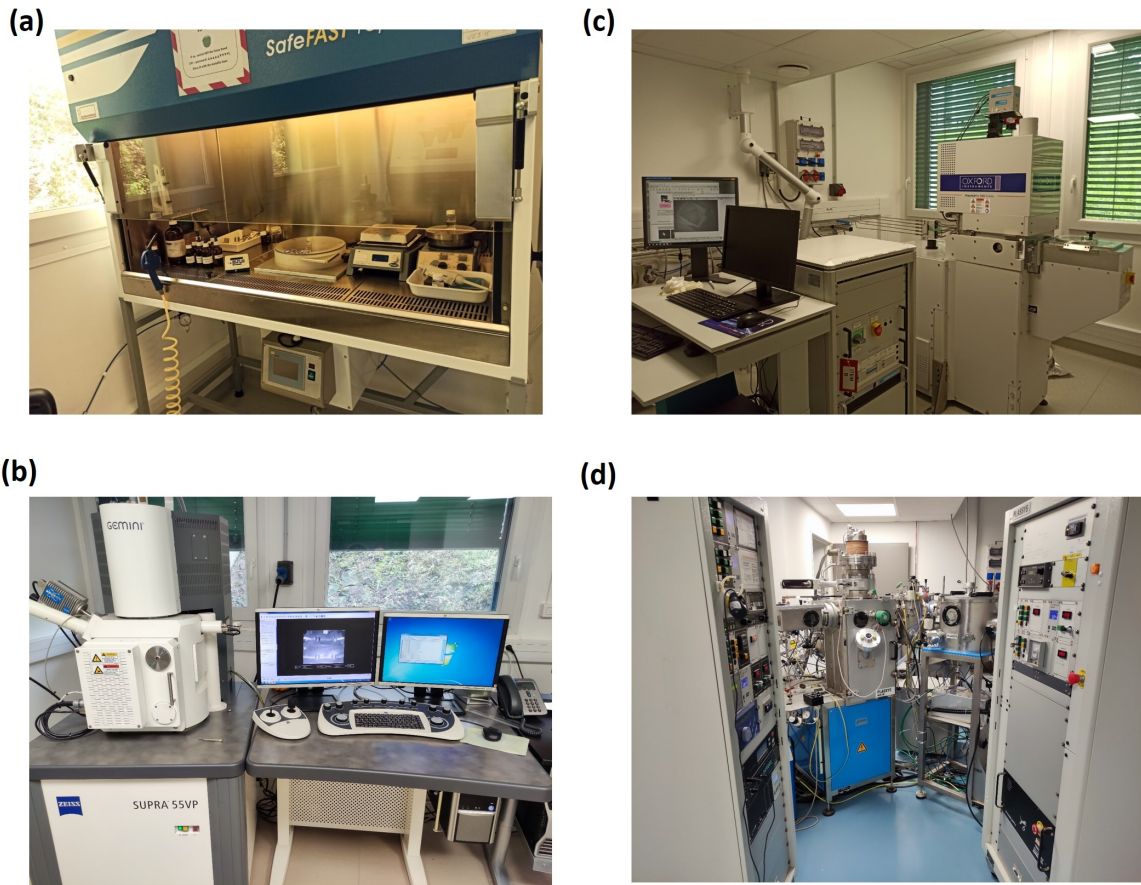
Fig. 3.8.1 (a) Spin Coater. (b) Lithography system. Scanning electron microscope Zeiss Supra55VP. (c) Reactive ion etching system. (d) Electron beam PVD and DC sputtering PVD system.
