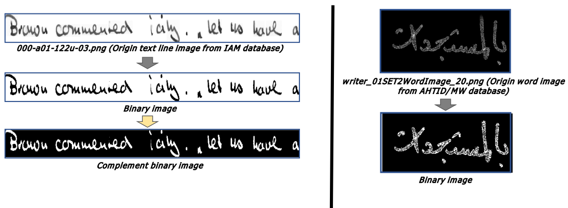
Figure 3.2: Example of binarization of handwritten samples from IAM (Marti and Bunke (2002)), and AHTID/MW (Mezghani et al. (2012)) databases.
