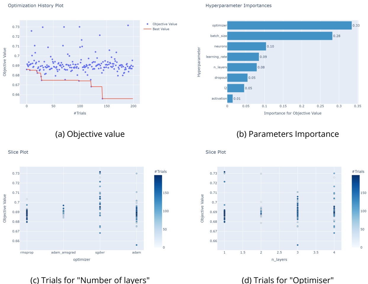
Figure 8.1: Illustration of the hyperparameter search using the Tree-Parzen algorithm with the optuna package in Python.
