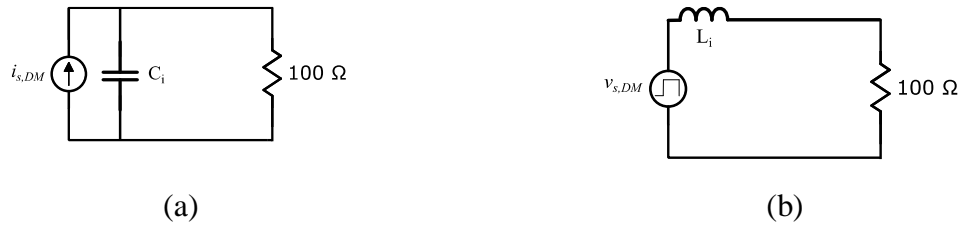
Figure 1.8 Simplified DM noise measured in simplified high-frequency equivalent system: (a) a noise source represented by a current flowing through a DC-link capacitor; (b) a noise source represented by voltage fluctuations coupled through an inductor, commonly observed in AC/DC converters. Content inspired by [39] and [41].
