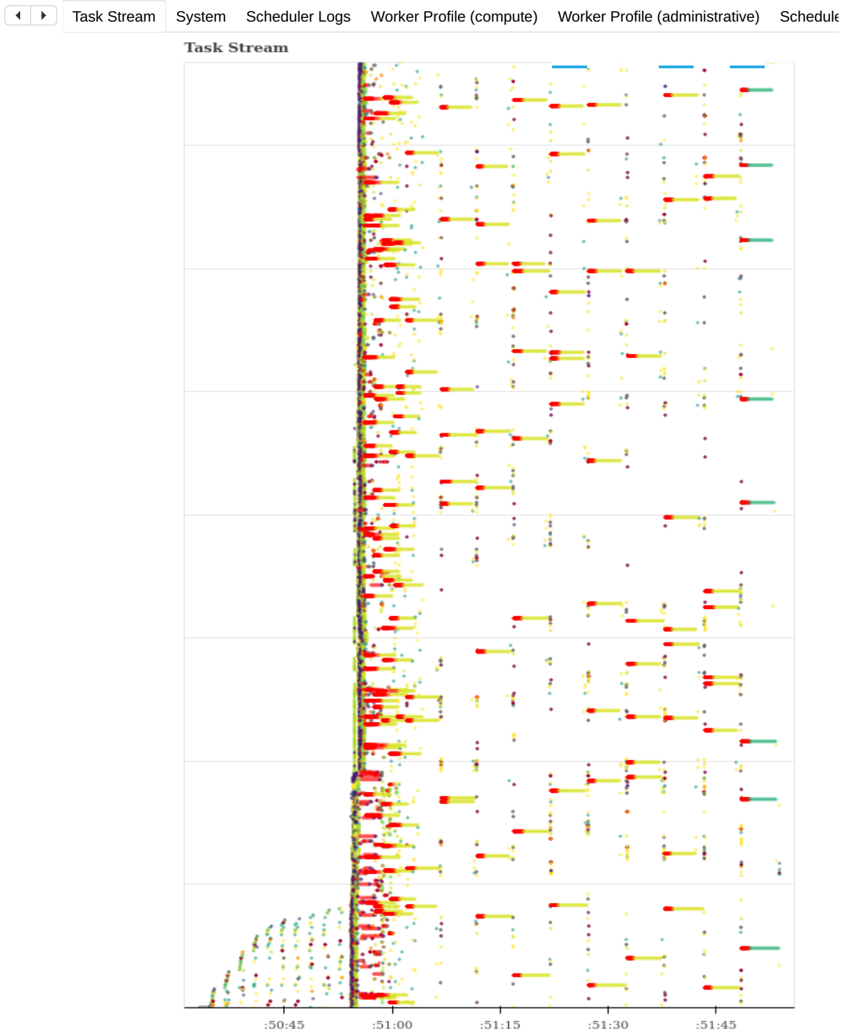
Figure 6.21: Task stream generated by Dask with in situ analytics enabled for the new IPCA, for 64 processes, 32 workers and 128 MiB per process. Number of tasks: 7090. Compute time: 837.69s. Deserialize time: 1.47s. Transfer time: 1354.78s.
