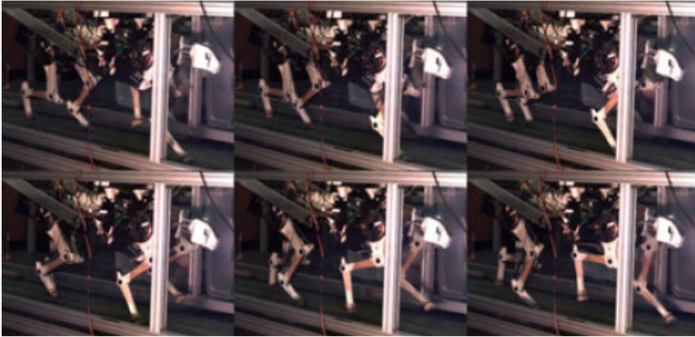
Figure 1.10: MIT Cheetah, running at 6 m/s [Seok et al., 2015]
