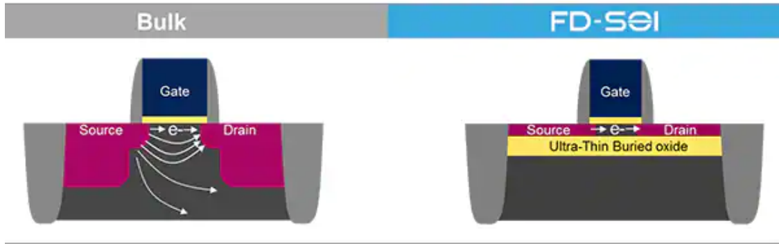
Figure 1.2: Bulk CMOS vs FD-SOI (Source: STMicroelectronics)
