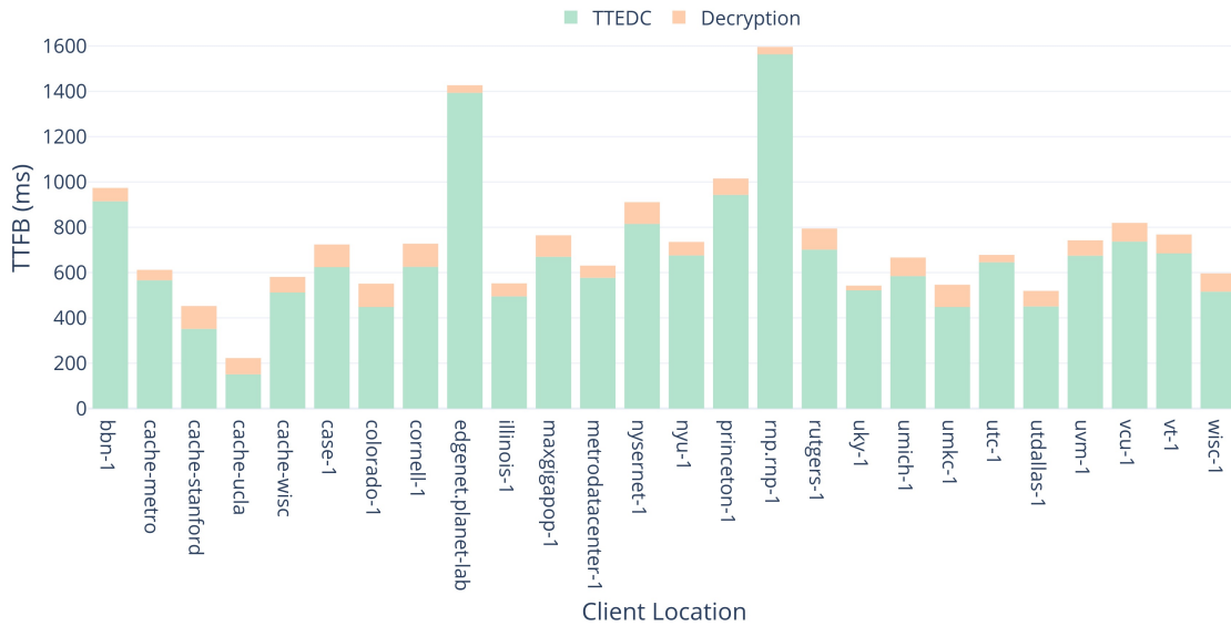
Figure 5.11: The implications of the decryption time on TTFB for the Los Angeles case.
