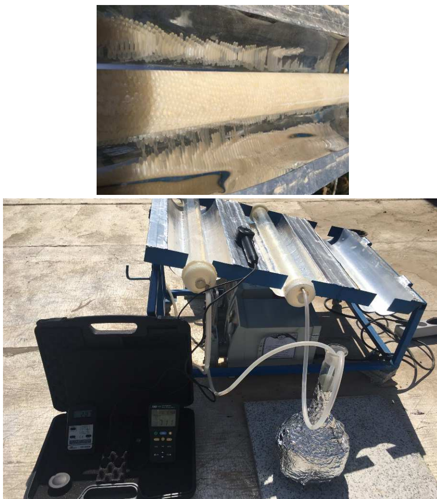
Figure 63. Photos of the CPC solar photo-reactor with its measurement equipment installed at the University of Isfahan, Iran.
