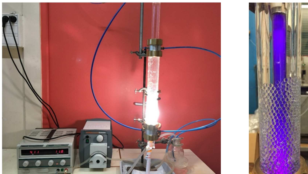
Figure 65. Photos of the lab-scale photoreactor with an artificial light installed at LSPM, France.
