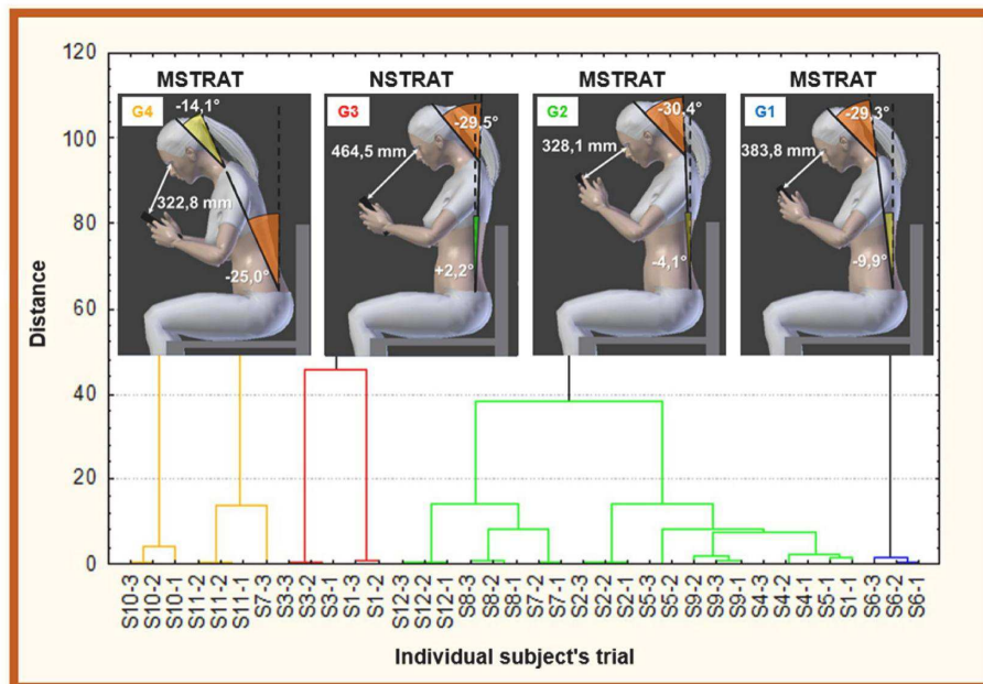
Fig. 4. Ward's minimum variance linkage dendrogram of the hierarchical cluster analysis of smartphone users while achieving the TEXT task under the SWT condition representing the four-cluster solution. Four groups are highlighted by blue color for Group 1 (G1), green color for Group 2 (G2), red color for Group 3 (G3) and orange color for Group4 (G4). Participant and trial numbers are indicated. Colored angular sectors represent are based on the RULA ergonomic table (McAtamney and Nigel Corlett, 1993). See Fig. 8 for color legend. (For interpretation of the references to color in this figure legend, the reader is referred to the Web version of this article).
