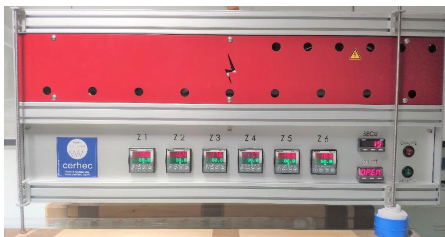
Figure II.4 Sublimation equipment with temperature gradients
