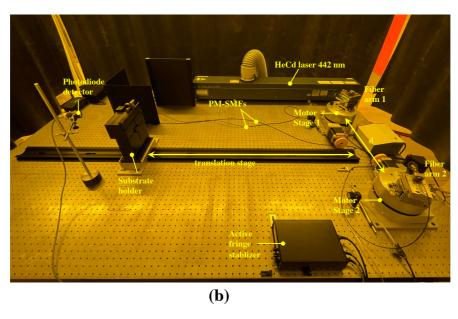
**Figure 2.11.** (a) The schematic sketch and (b) a Photograph of the LIL setup (Nano Saint-Etienne platform, LabHC).
