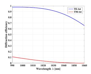
**Figure 2.21.** Recalculated DE for TE and TM in -1<sup>st</sup> order for GWS parameter obtained by fabrication process with grating period 623.5 nm, grating depth of 80 nm, and Duty Cycle of 30%. DE at 1030 nm for TE -1<sup>st</sup> order is 91.5%
