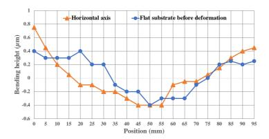
Figure 3.12. Optical profilometry measurement data of deformed 4-inch silicon wafer after the vacuum treatment for 30 minutes. The orange plot ( $\blacktriangle$ ) is the flatness of the wafer measured along the horizontal axis with a maximum deviation of 1.17  $\mu$ m. The blue plot ( $\bullet$ ) is the flatness of the wafer along the horizontal axis with a maximum deviation of 0.80  $\mu$ m.
