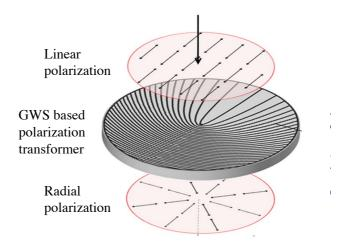
**Figure 1.16.** Transformation of linear polarization to radial polarization using segmented GWS [132].
