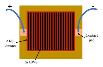
**Figure 1.11.** Schematic in the top view of GWS used in thermos-optic tunable filtering by Joule heating arrangement.
