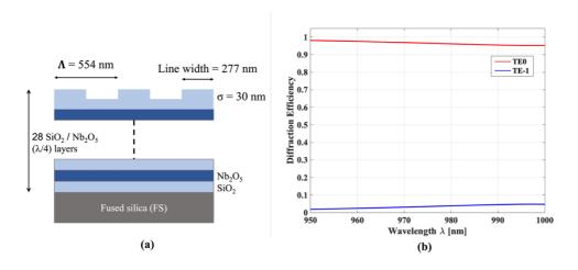
**Figure 2.3.** Design of low-index GWS for A3 application, (a) sketch with design parameters. (b) The calculated DE plot for TE at  $0^{th}$  and  $-1^{st}$  order with TE<sub>0</sub>>92.5% and TE<sub>-1</sub><7.5% at 976 nm.
