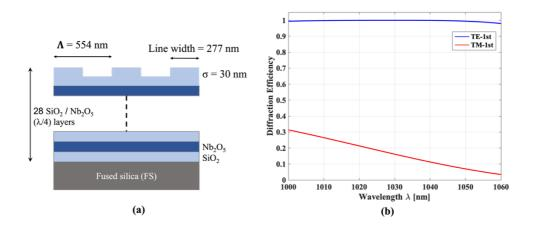
**Figure 2.7.** Design of high-index GWS for A4 application, (a) sketch with design parameters. (b) The calculated DE plot for TE and TM -1<sup>st</sup> order with TE<sub>-1</sub> >99.9% at 1030 nm.
