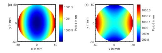
**Figure 3.3.** Calculated period distributions with the equations from Bienert et al. [165]. The color scale indicates the period. (a): Flat substrate. (b): Curved substrate with a radius of curvature of 1000 mm.
