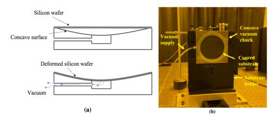
**Figure 3.4.** (a) Sketch of the bending process of a silicon wafer by concave vacuum chuck. (b) Image of concave vacuum chuck mounted on substrate holder stand with silicon wafer curved using vacuum supply.
