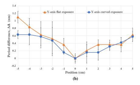
**Figure 3.7.** A measured period variation along the x-axis (a) and y-axis (b) on the silicon wafer exposed by two spherical waves at the central period of 1000 nm. The orange plot ( $\triangle$ ) is the period variation on the flat exposed substrate. The blue plot ( $\bullet$ ) is the period variation on the curved exposed substrate. The error bars indicate the uncertainty in the diffraction angle measurements.
