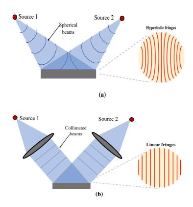
**Figure 1.21.** Interference fringes formed two different LIL setups with, (a) Two-spherical beams resulting in the hyperbolic fringe patterning. (b) Two collimated beams resulted in the near-linear fringe patterning.
