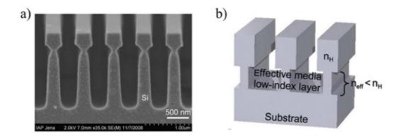
**Figure 1.12.** (a) SEM image of a T-like GWS structure with silicon on silica substrate [112]. (b) Schematic of a single silicon crystal GWS mirror [113].
