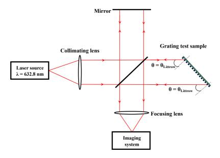
Figure. 3.13. The working setup of adaptive wavefront interferometry.
