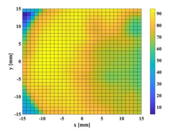
**Figure 2.20.** The measured spatial DE in TE -1<sup>st</sup> order of 2-inch GWS with a grating period of 623.5 nm and grating depth of 80 nm with a Duty Cycle of 30%.
