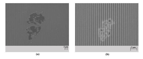
**Figure 2.27(a-b).** SEM image of GWS fabricated and etched in direct LIL fabrication process flow with defect spots with spot sizes from 2  $\mu$ m to 10  $\mu$ m.
