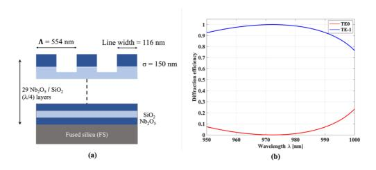
**Figure 2.5.** Design of high-index GWS for A3 application, (a) sketch with design parameters. (b) The calculated DE plot for TE at  $0^{th}$  and  $-1^{st}$  order with TE<sub>-1</sub>>99.9% at 976 nm.
