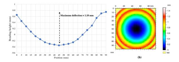
**Figure 3.11.** Optical profilometry (a) measurement data of deformed 4-inch silicon wafer during the vacuum treatment. (b) Surface topography of the wafer during the vacuum treatment. The maximum deflection at the center of the wafer is 1.10 mm.
