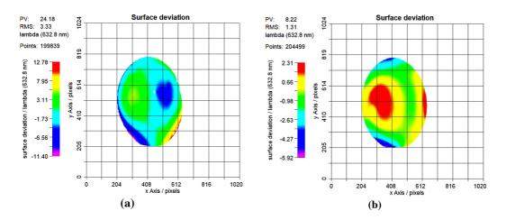
**Figure 3.14.** The surface deviation of the 4-inch substrate at the central period of 1000 nm was recorded by wavefront aberration measurement using a laser at  $\lambda = 632.8$  nm (a) For flat exposed grating, P-V is 24.18 $\lambda$ , and the RMS value is 3.33 $\lambda$ . (b) For curved exposed grating, P-V is 8.22 $\lambda$ , and the RMS value is 1.31 $\lambda$ .
