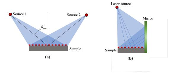
**Figure 1.20.** LIL setups with interferometry arrangement. (a) Two-beam LIL interferometer, (b) Single-beam interferometer (Lloyd's interferometer).
