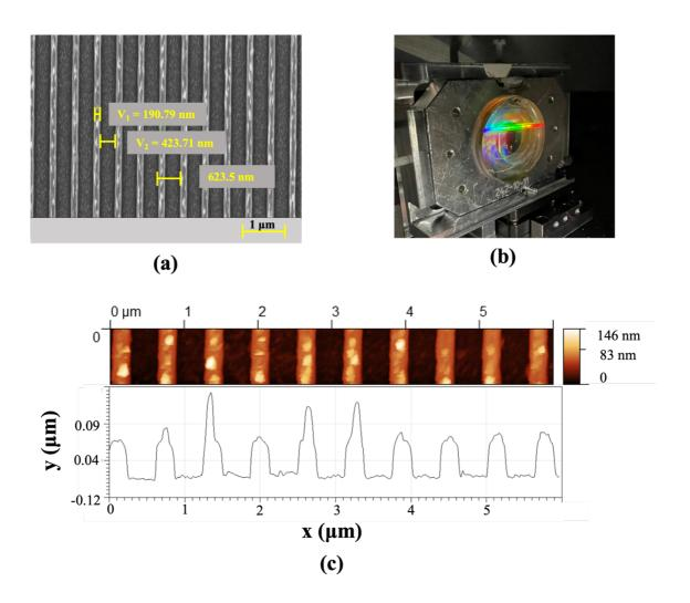
**Figure 2.15.** (a) SEM image (b) Photograph, and (c) AFM data and grating profile of Nb<sub>2</sub>O<sub>5</sub> etched grating surface on 2-inch multilayer substrate for A4 application.
