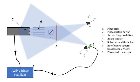
Figure 1.23. Schematic of active fringe stabilization setup.
