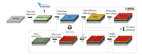
**Figure 2.10.** Complete fabrication process flow of grating with LIL direct patterning technique. The multilayer deposition (a) was carried out at Institut Fresnel (IF) by ESR 6, France. The process of BARC and photoresist deposition (b-c) and LIL patterning and development of photoresist gratings structures (d) are performed at Hubert Curien laboratory (LabHC), France. The etching process (f-g) is performed at the University of Eastern Finland (UEF) with the help of ESR 5, Finland.
