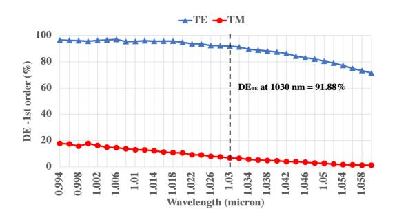
**Figure 2.19.** The measured DE of TE and TM -1<sup>st</sup> orders of GWS with a grating period of 623.5 nm and grating depth of 80 nm with a Duty Cycle of 30%.
