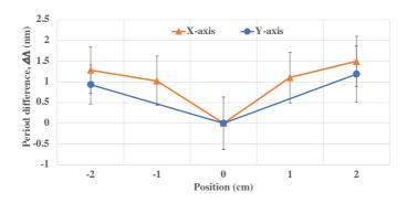
Figure 2.25. A measured period variation along the 2-inch Si master grating A3 application with a grating period of 556 nm at the substrate's center. The orange plot ( $\triangle$ ) is the period variation along the x-axis. The blue plot ( $\bullet$ ) is the period variation along the y-axis. The error bar reflects the uncertainty in the diffraction angle measurements.
