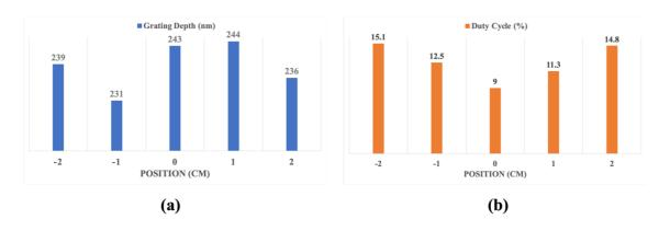
**Figure 2.24.** Variation in grating depth and Duty Cycle on 2-inch Si etched master grating with grating depth varying by 13 nm and Duty Cycle varying by 7% along the central *x*-axis for A3 applications.
