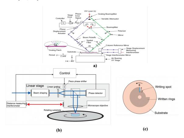
**Figure 1.18.** (a) Schematic of the SBIL system [138] (b) Illustrates the SBIL process setup for patterning circular gratings. (c) The substrate stage is rotated, resulting in the ring patterns of gratings [142].
