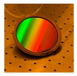
**Figure 3.5.** Photograph of fabricated photoresist grating on a 4-inch silicon wafer of thickness 525 μm using concave vacuum chuck holder by two-spherical-beam 442 nm LIL setup with an exposure time of 3 minutes and developing time of 5 seconds at 21°C.
