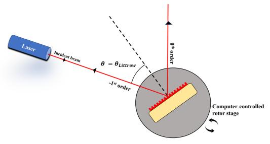
Figure 3.6. Schematic of diffraction period measurement at Littrow configuration.
