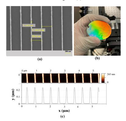
**Figure 2.23.** (a) SEM image, (b) Photograph, and (c) AFM data and grating profile of Si etched master grating with a grating depth of 243 nm at the center of the substrate and Duty Cycle of 9% on 2-inch Si for A3 application.
