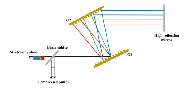
**Figure 1.13.** The configuration of pulse compression using G<sub>1</sub>-G<sub>2</sub> GWS pair.
