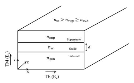
Figure 1.6. Schematic of dielectric planar waveguide [63].
