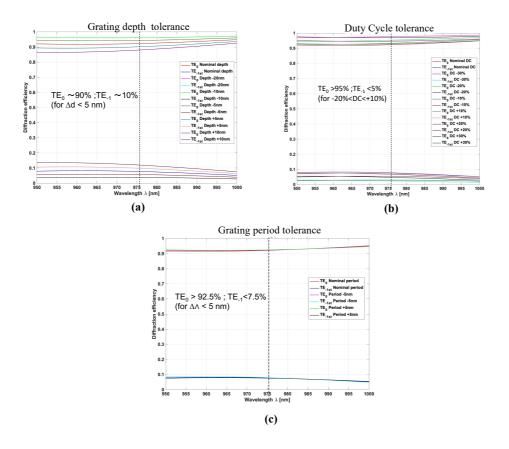
**Figure 2.4.** Simulated tolerance of low-index GWS for A3 application, (a) Grating depth tolerance for variation from -20 nm to +10 nm. (b) Duty Cycle tolerance for variation from -30 % to +30 %. (c) Grating period tolerance for variation from -5 nm to +5 nm.
