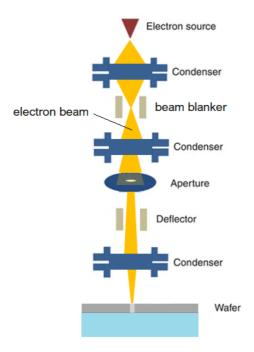
**Figure 1.17.** Schematic illustration of the EBL process. The electron beam is focused on electron sensitive resist layer for the patterning of nanostructures.
