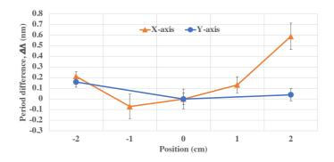
**Figure 2.17.** A measured period variation along the 2-inch high index GWS for A4 application with a grating period of 623 nm at the substrate's center. The orange plot ( $\blacktriangle$ ) is the period variation along the *x*-axis. The blue plot ( $\bullet$ ) is the period variation along the *y*-axis. The error bar reflects the uncertainty in the diffraction angle measurements.
