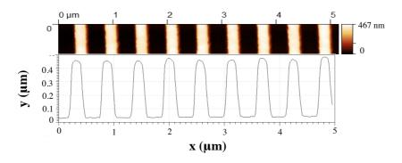
**Figure 2.22.** AFM data and grating profile of photoresist grating surface on a 2-inch Si substrate to develop master gratings for A3 application.
