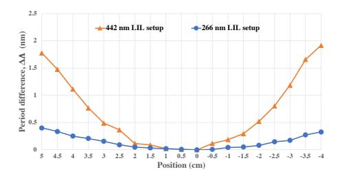
**Figure 3.9.** A measured period variation on the x-axis of the flat exposed substrate with two LIL optical set-ups for the grating period of 500 nm. The orange plot ( $\triangle$ ) is the period variation on the flat exposed substrate using a 442 nm LIL setup. The blue plot ( $\bullet$ ) is the period variation on the flat exposed substrate using a 266 nm LIL setup.
