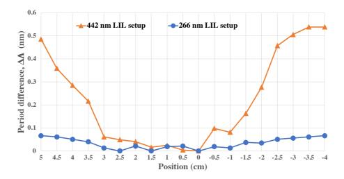
**Figure 3.10.** A measured period variation on the x-axis of the curved exposed substrate with two LIL optical set-ups for the grating period of 500 nm. The orange plot (▲) is the period variation on the curved exposed substrate using a 442 nm LIL setup. The blue plot (•) is the period variation on the curved exposed substrate using a 266 nm LIL setup.
