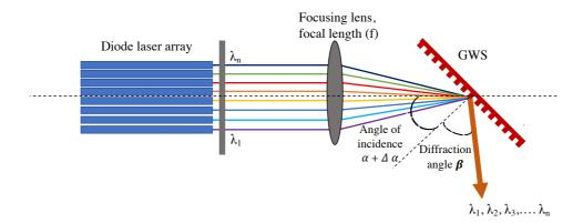
**Figure 1.14.** Schematic configuration of wavelength multiplexing of diode laser array by using GWS to combine the wavelengths  $(\lambda_1, \lambda_2, \lambda_3, ...., \lambda_n)$  from n number of diode lasers using a focusing lens.
