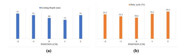
**Figure 2.16.** Variation in grating depth and Duty Cycle on 2-inch Nb<sub>2</sub>O<sub>5</sub> etched multilayer GWS with grating depth varying by 24 nm and Duty Cycle varying by 9% along the central *x*-axis for A4 application.
