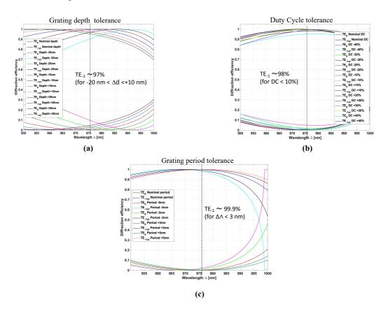
**Figure 2.6.** Simulated tolerance of high-index GWS for A3 application, (a) Grating depth tolerance for variation from -30 nm to +30 nm. (b) Duty Cycle tolerance for variation from -40 % to +40 %. (c) Grating period tolerance for variation from -5 nm to +5 nm.
