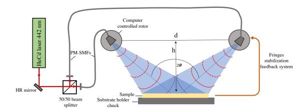
**Figure 1.22.** Schematic configuration of the two-spherical beam LIL setup used for the grating patterning GWS and Si masters (Nano Saint-Etienne platform, France). The spherical-beam interference fringes are of hyperbolic shapes due to the fringe inclination, and the interference angle changes when moved away from the center of the substrate (h).
