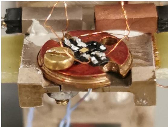
Fig. 2.17: Close picture of the set-up for ac specific heat.
