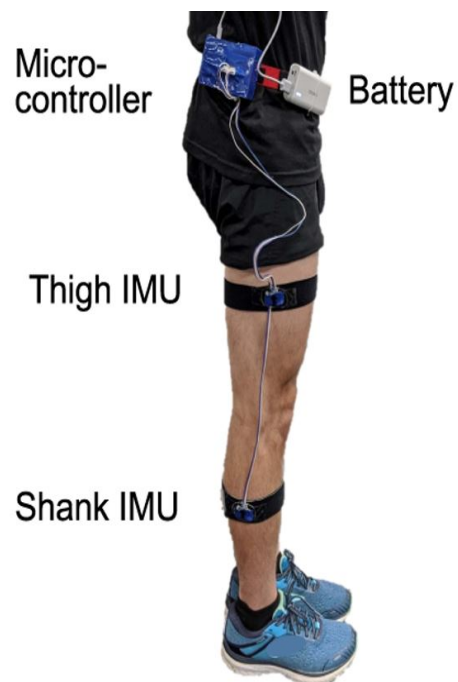
Figure 1.3 – Example of IMUs Used for Gait Analysis
