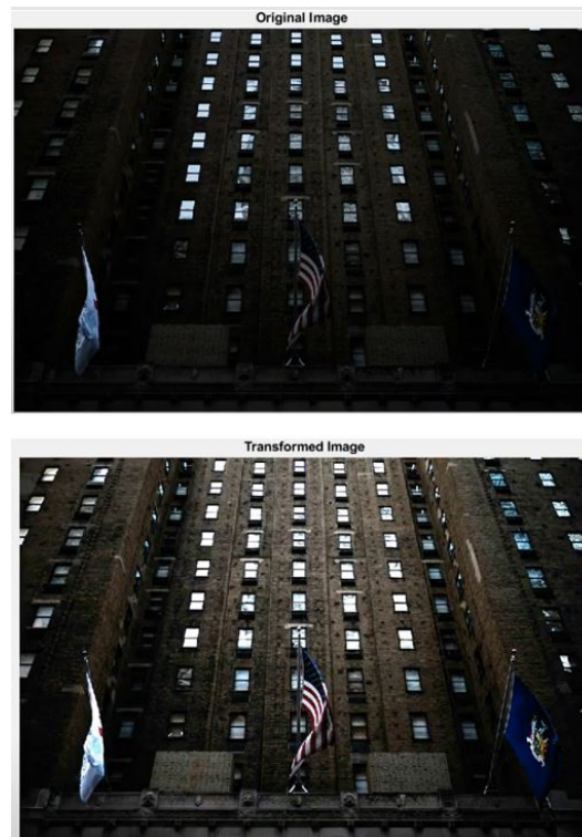
Figure 4.12 – An Example of a Log Transformation on a Colored Image
