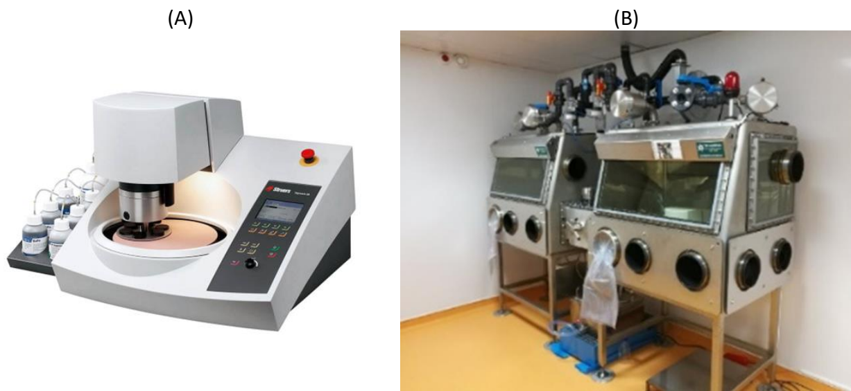
Figure 177: (A) The Struers Tegramin Polisher and (B) the polisher inside the glovebox at the GENESIS platform.
